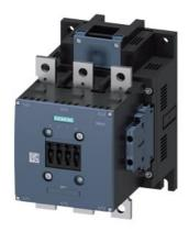
power contactor, AC-3 265 A, 132 kW / 400 V AC (50-60 Hz) / DC operation 500-550 V AC/DC auxiliary contacts 2 NO + 2 NC 3-pole, frame size S10 busbar connections drive: conventional screw terminal
