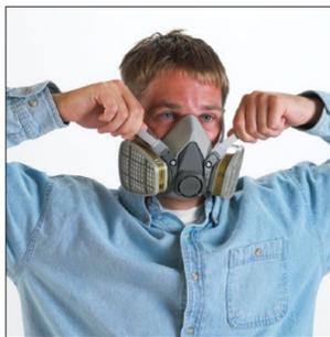
Adjust strap tension to achieve a secure fit. Pull the ends of the straps to adjust the tightness beginning with the adjustment points at the top of the respirator and then moving to the adjustment points at the back of the neck. Do not over-tighten. Strap tension may be decreased by pushing out on back side of buckles.
