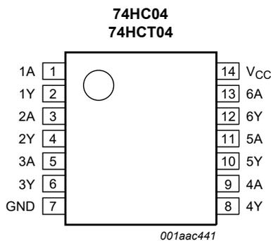
Fig. 4. Pin configuration SOT108-1 (SO14) and SOT402-1 (TSSOP14)
