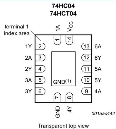
(1) This is not a ground pin. There is no electrical or mechanical requirement to solder the pad. In case soldered, the solder land should remain floating or connected to GND
