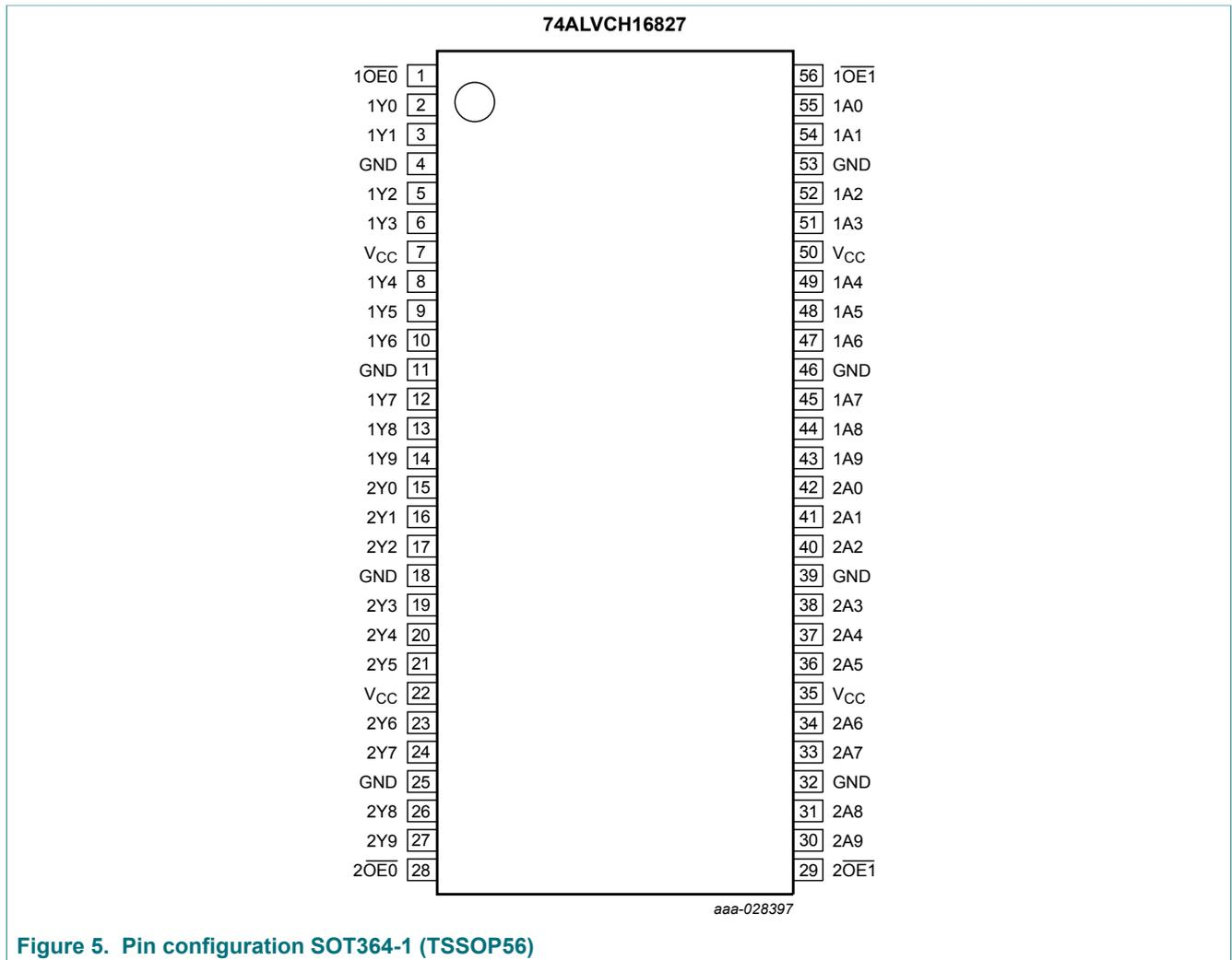
Figure 5. Pin configuration SOT364-1 (TSSOP56)
