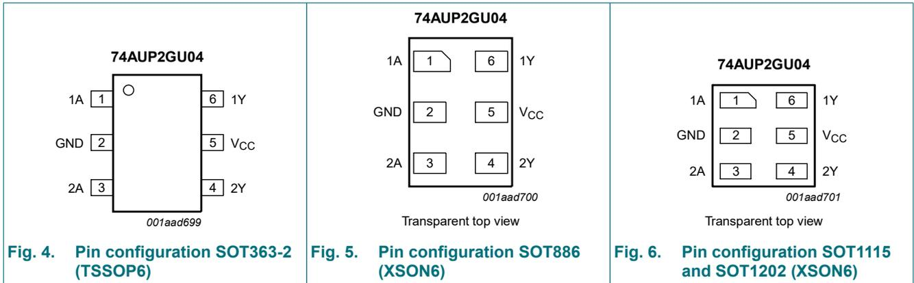
Fig. 4. Pin configuration SOT363-2 (TSSOP6)
