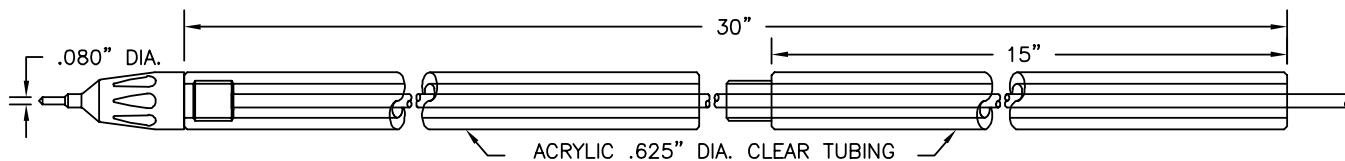
**CONSTRUCTION:** .080" (2.03mm) 1/4-32 threaded assembly, solderless connection. Plated brass tip. Clear acrylic probe unscrews into two 15" (381 mm) pieces for convenient storage. Available with factory assembled leads only. 18 AWG PVC wire.
