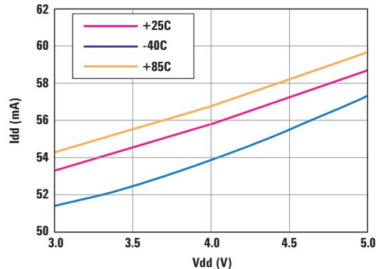
Figure 12. Bias current over temperature.
