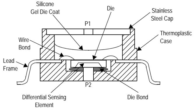
**Figure 4. SOP Package — Cross-Sectional Diagram (Not to Scale)**
