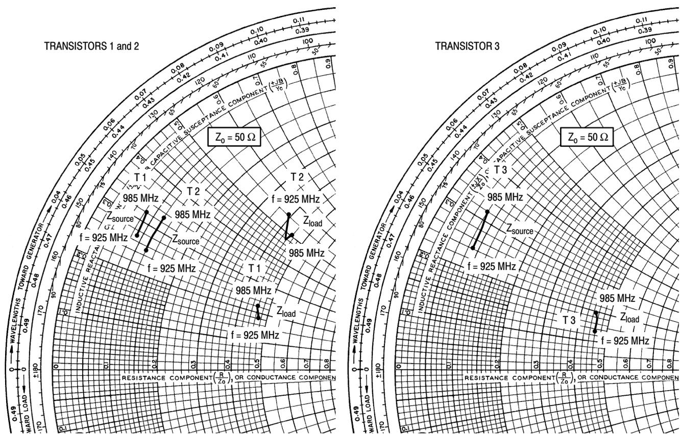
$V_{DD} = 26\text{ V}$ ,  $I_{DQ} = 25\text{ mA}$ ,  $P_{out} = 2\text{ W PEP}$
