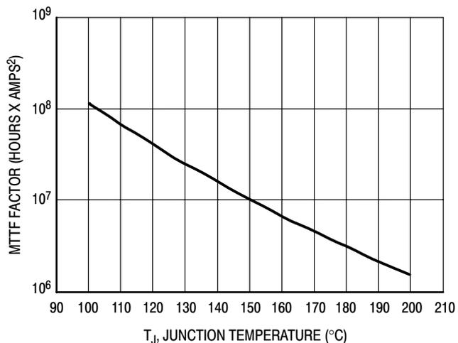
This above graph displays calculated MTTF in hours x ampere<sup>2</sup> drain current. Life tests at elevated temperatures have correlated to better than ±10% of the theoretical prediction for metal failure. Divide MTTF factor by I<sub>D</sub><sup>2</sup> for MTTF in a particular application.
