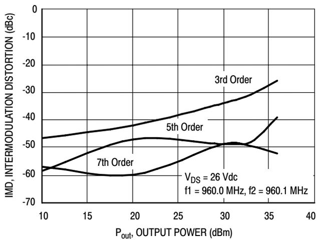
**Figure 8. Intermodulation Distortion Products versus Output Power**
