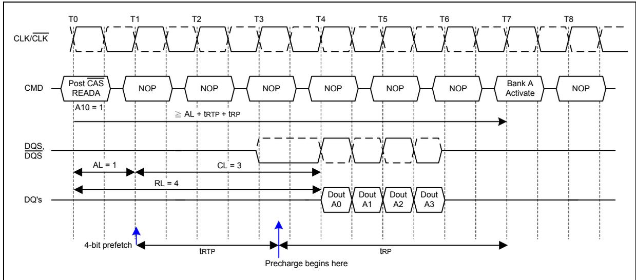
**10.25 Burst read with Auto-precharge followed by an activation to the same bank (tRC Limit): RL=5 (AL=2, CL=3, internal tRCD=3, BL=4,  $t_{RTP} \leq 2\text{clks}$ )**
