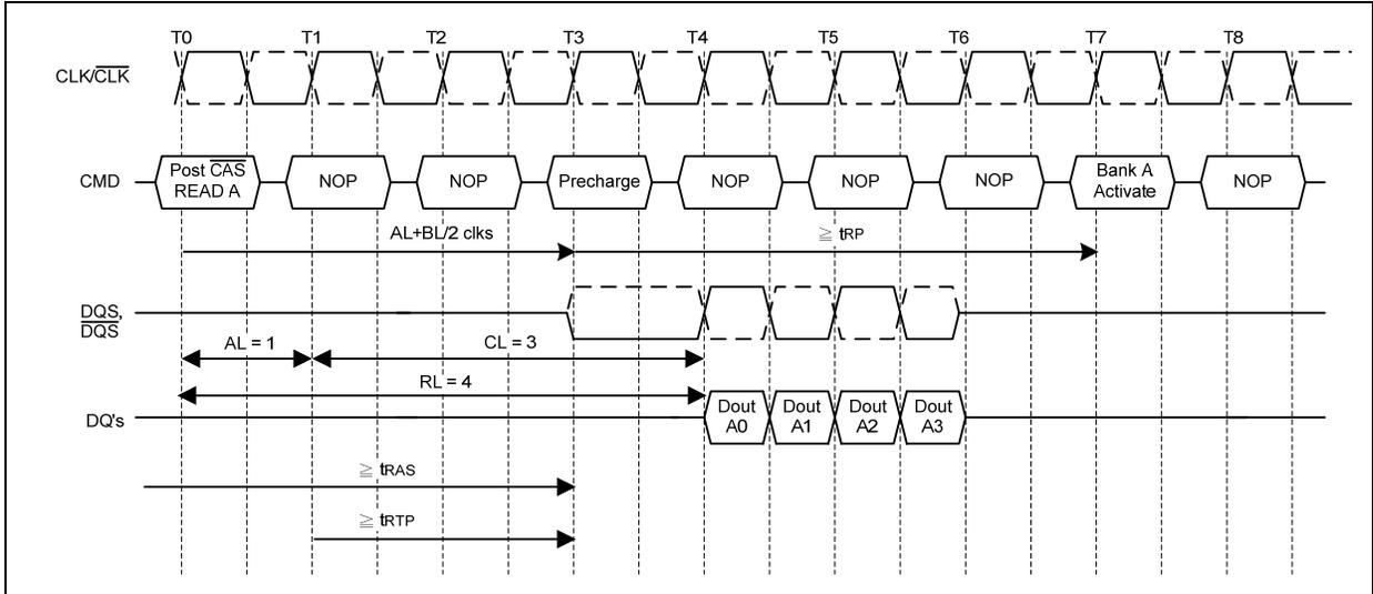
**10.17 Burst read operation followed by precharge: RL=4 (AL=1, CL=3, BL=8,  $t_{RTP} \leq 2\text{clks}$ )**
