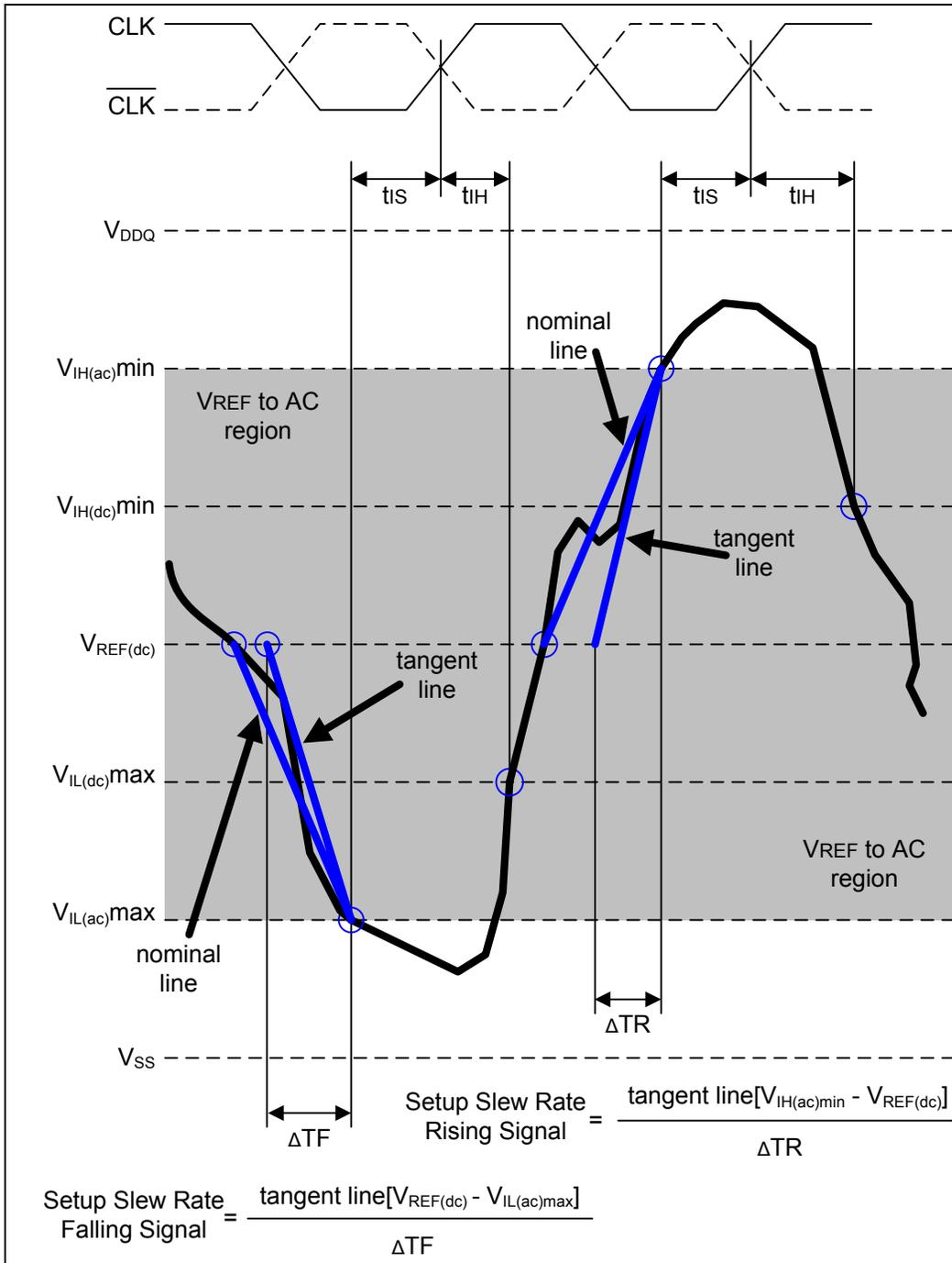
Figure 21 —Illustration of tangent line for t<sub>s</sub>
