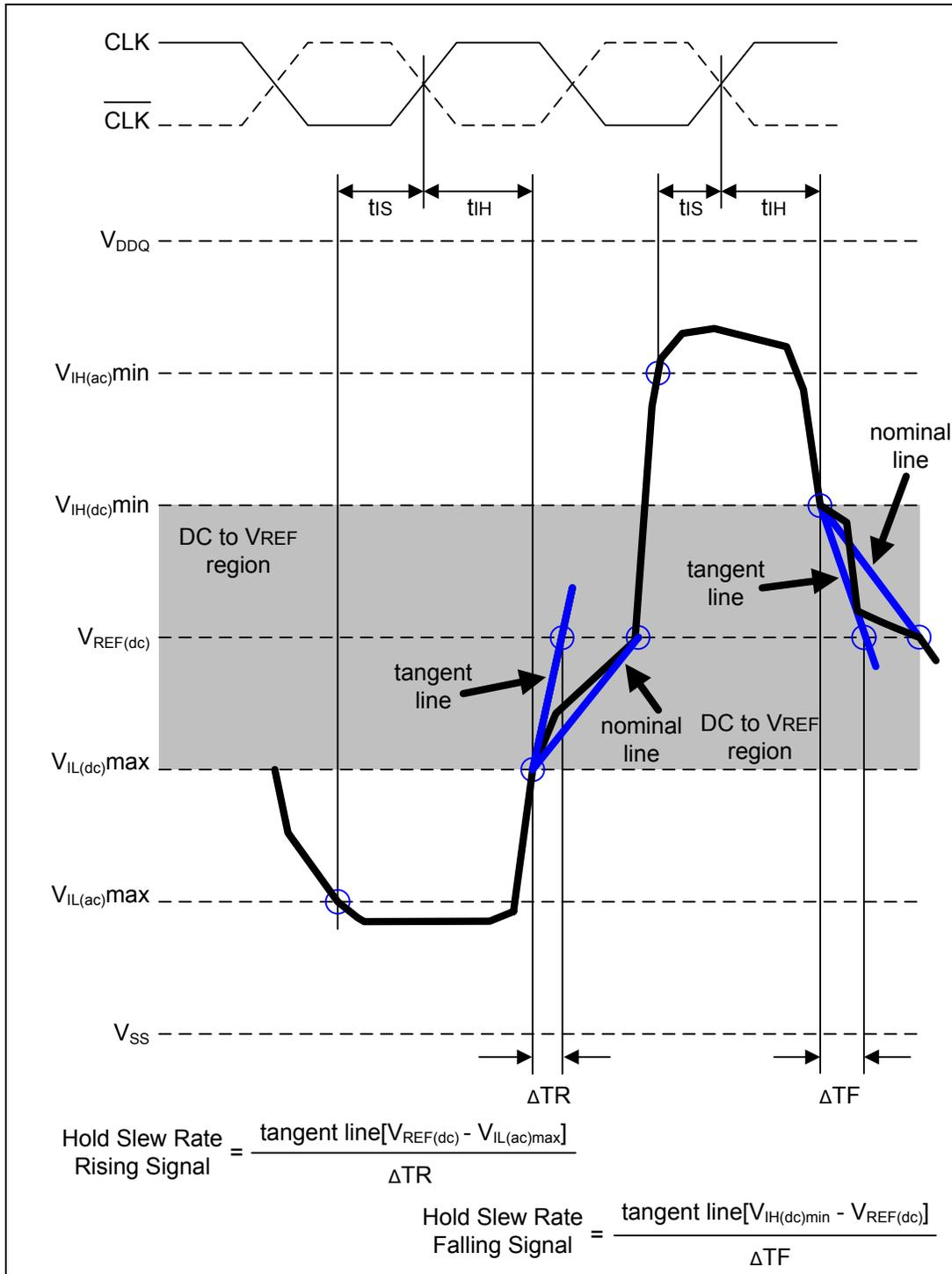
Figure 23 —Illustration of tangent line for tIH
