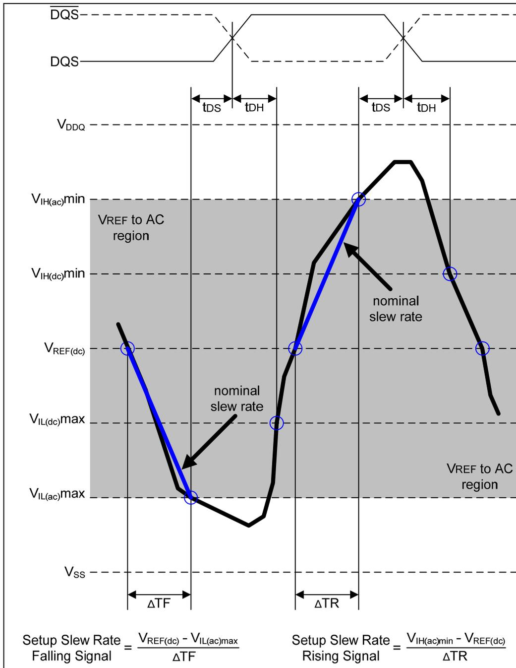
Figure 24 —Illustration of nominal slew rate for t<sub>DS</sub> (differential DQS,  $\overline{DQS}$ )
