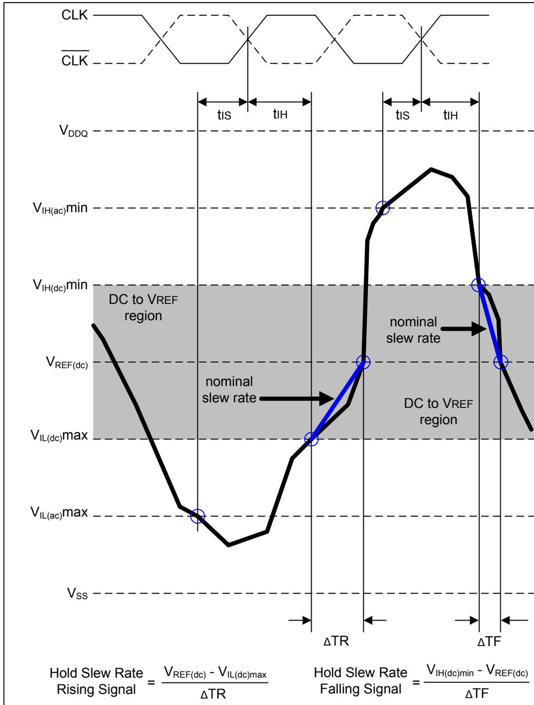
Figure 22 —Illustration of nominal slew rate for t<sub>H</sub>
