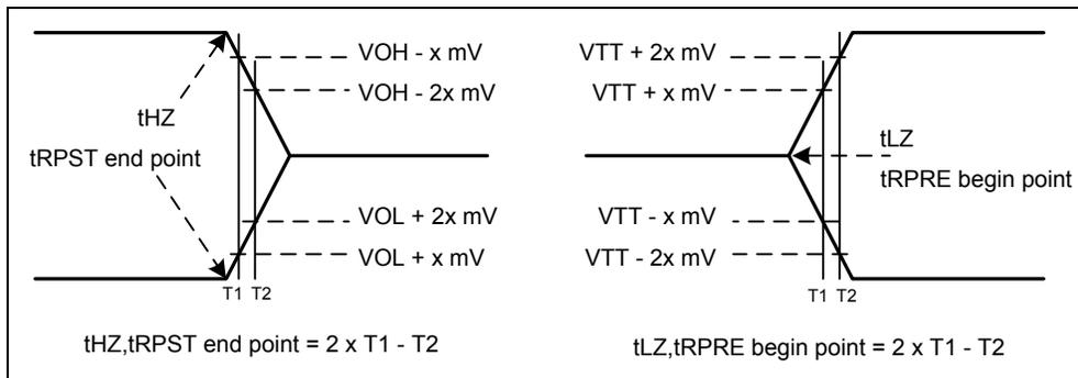
**Figure 18 — Method for calculating transitions and endpoints**
