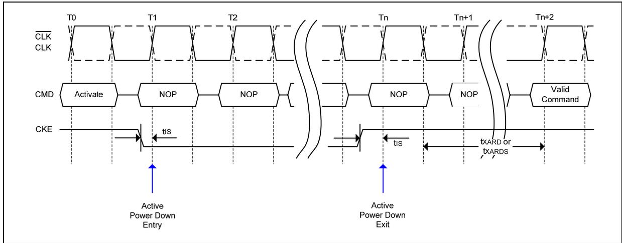
**10.31 Precharged Power Down Mode Entry and Exit Timing**
