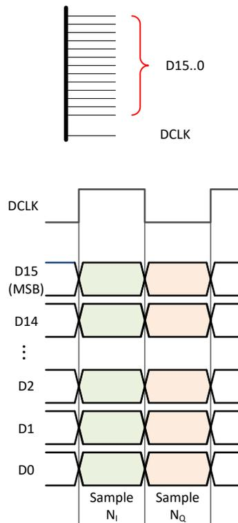
**Figure 8-30. Output Data Format in Complex Decimation**
