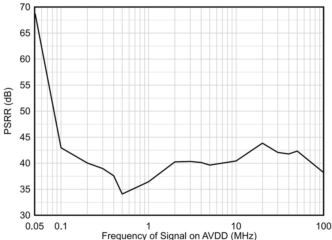
**Figure 9-6. Power supply rejection ratio (PSRR) vs frequency**
