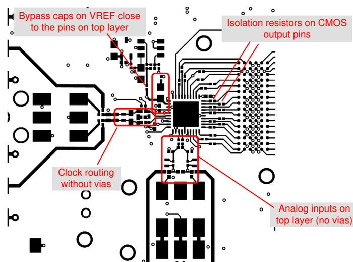
Figure 9-9. Layout example: top layer of ADC3544 EVM
