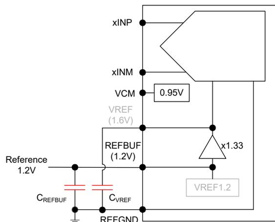
**Figure 8-13. External 1.2 V reference using internal reference buffer**
