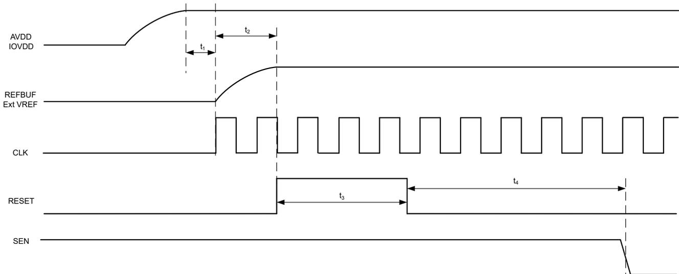
**Figure 9-5. Initialization of serial registers after power up**
