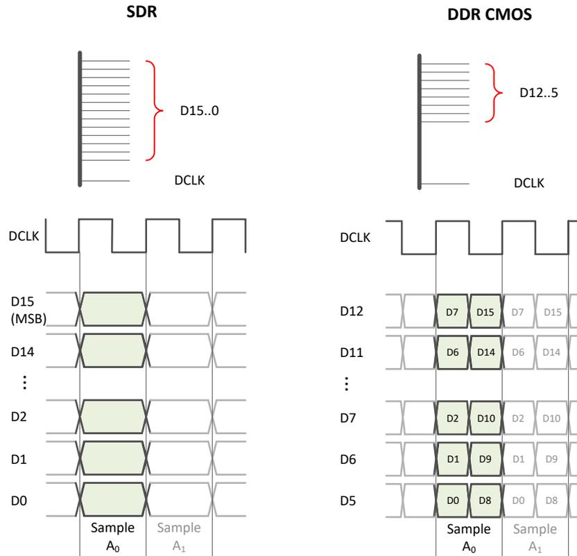
**Figure 8-31. Output Data Format in Real Decimation**
