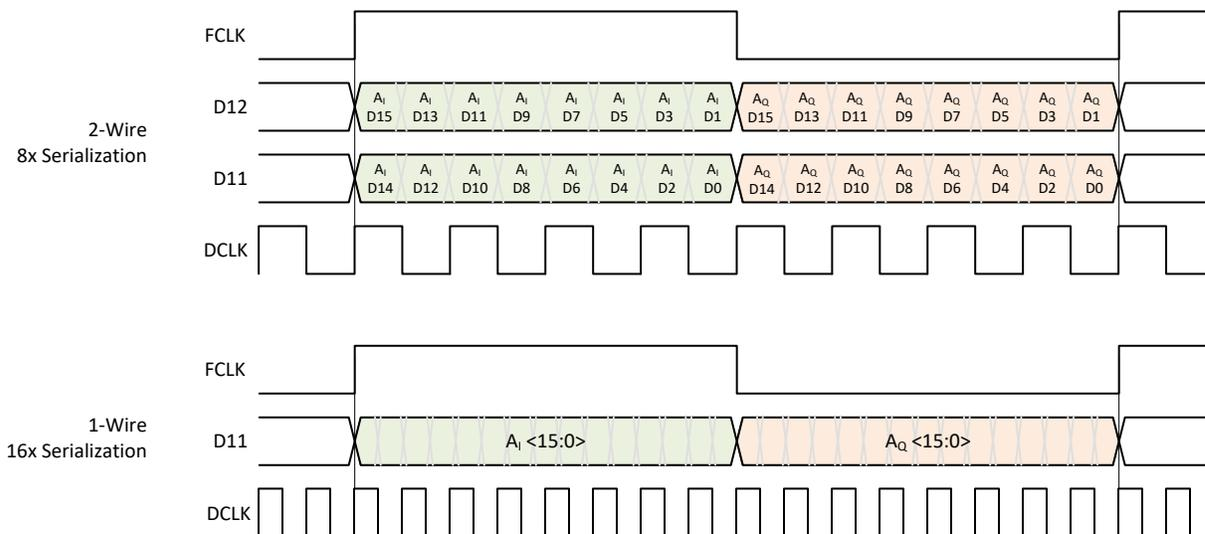
**Figure 8-32. Output Data Format in Complex Decimation**
