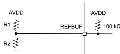
**Figure 8-44. Configuration of external voltage on REFBUF pin**
