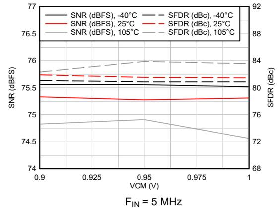
**Figure 6-18. AC Performance vs VCM vs Temperature**
