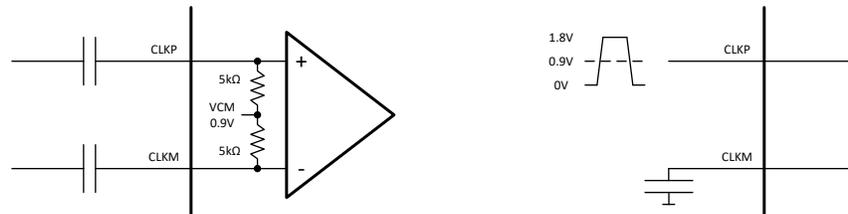
**Figure 8-9. External and internal connection using differential (left) and single ended (right) clock input**
