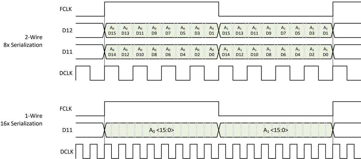
**Figure 8-33. Output Data Format in Real Decimation**
