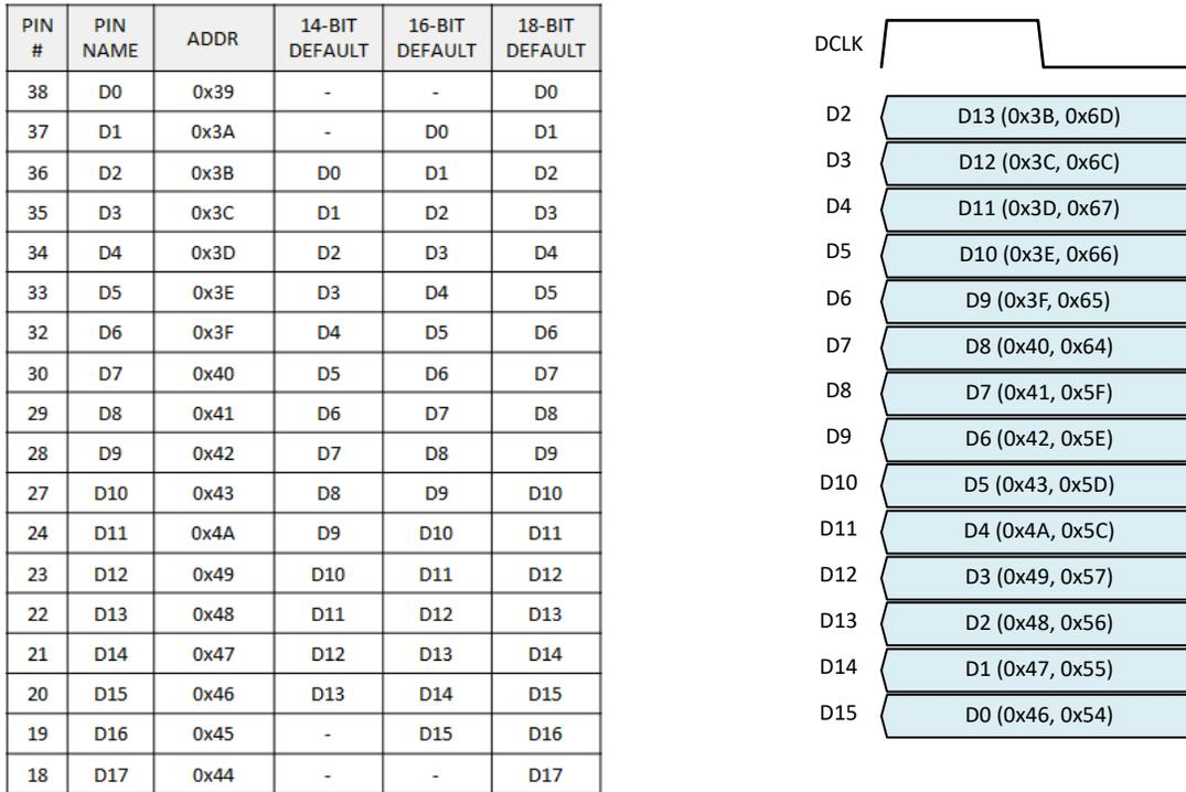
**Figure 8-37. SDR output mapping (left) and example (right)**
