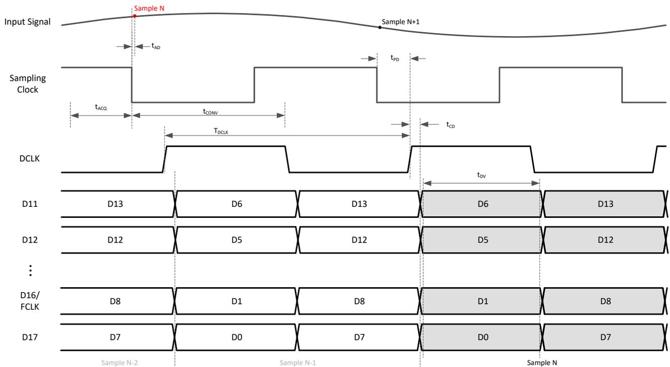
**Figure 7-2. Timing Diagram: DDR CMOS (default bit mapper)**
