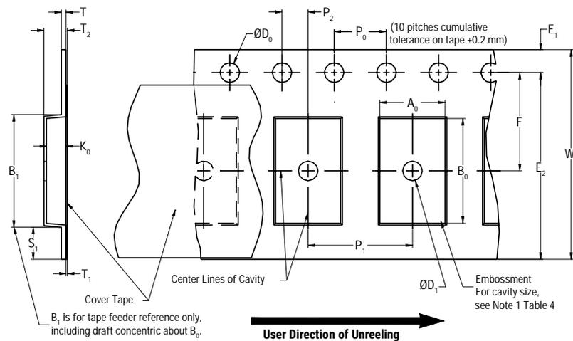
**Figure 2 – Punched (Paper) Carrier Tape Dimensions**
