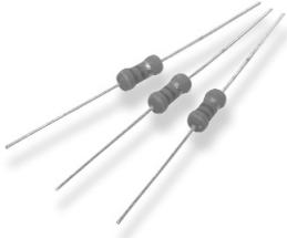
The resistive element comprises a resistive film sputtered onto a ceramic element. Metal end caps are force fitted to the element prior to spiralling. Tinned copper lead wires are welded to the end caps and the components are then coated with four layers of a flame-proof cement. All resistors are tested for value and tolerance. The technology allows the manufacture of custom fusible characteristics.
