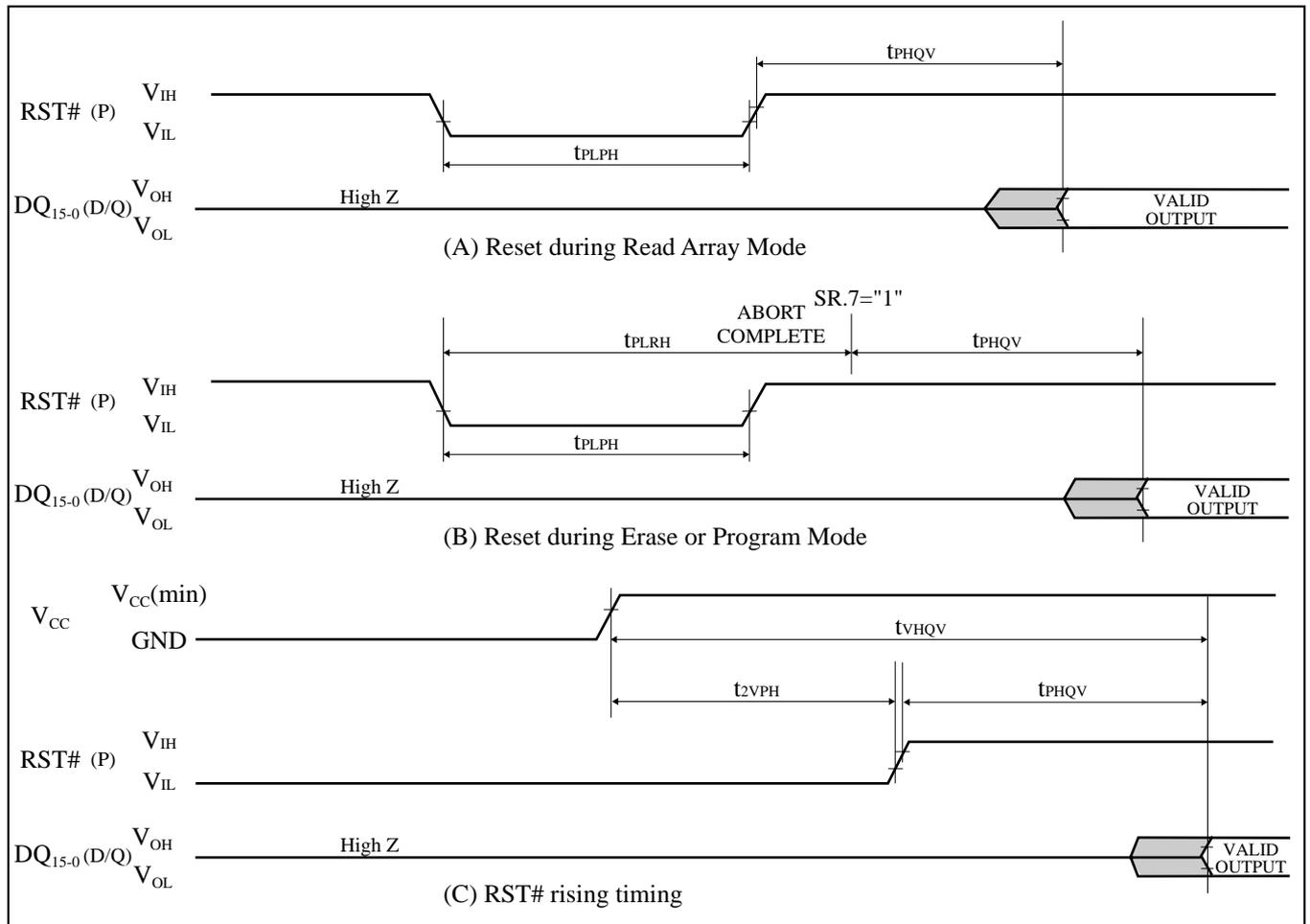
Figure 8. AC Waveform for Reset Operations
