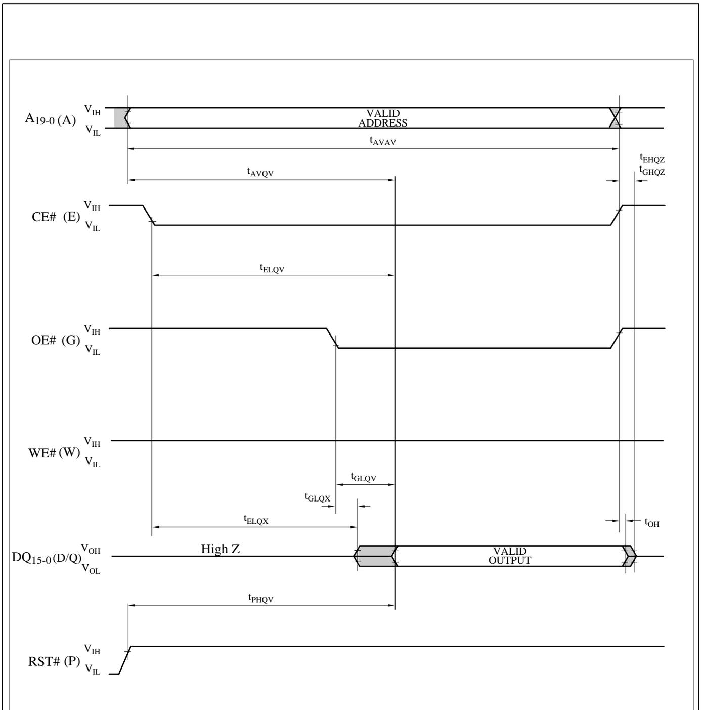
Figure 6. AC Waveform for Read Operations
