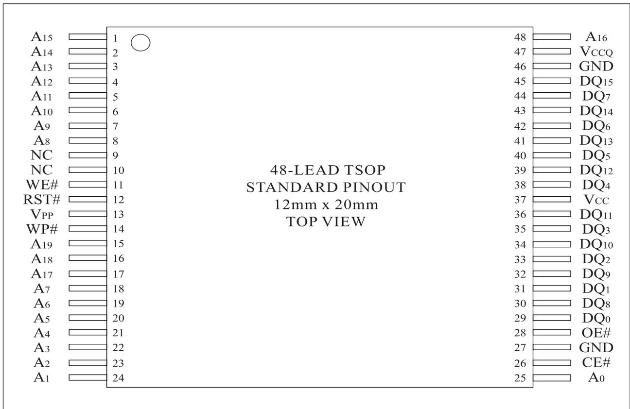
Figure 1. 48-Lead TSOP (Normal Bend) Pinout
