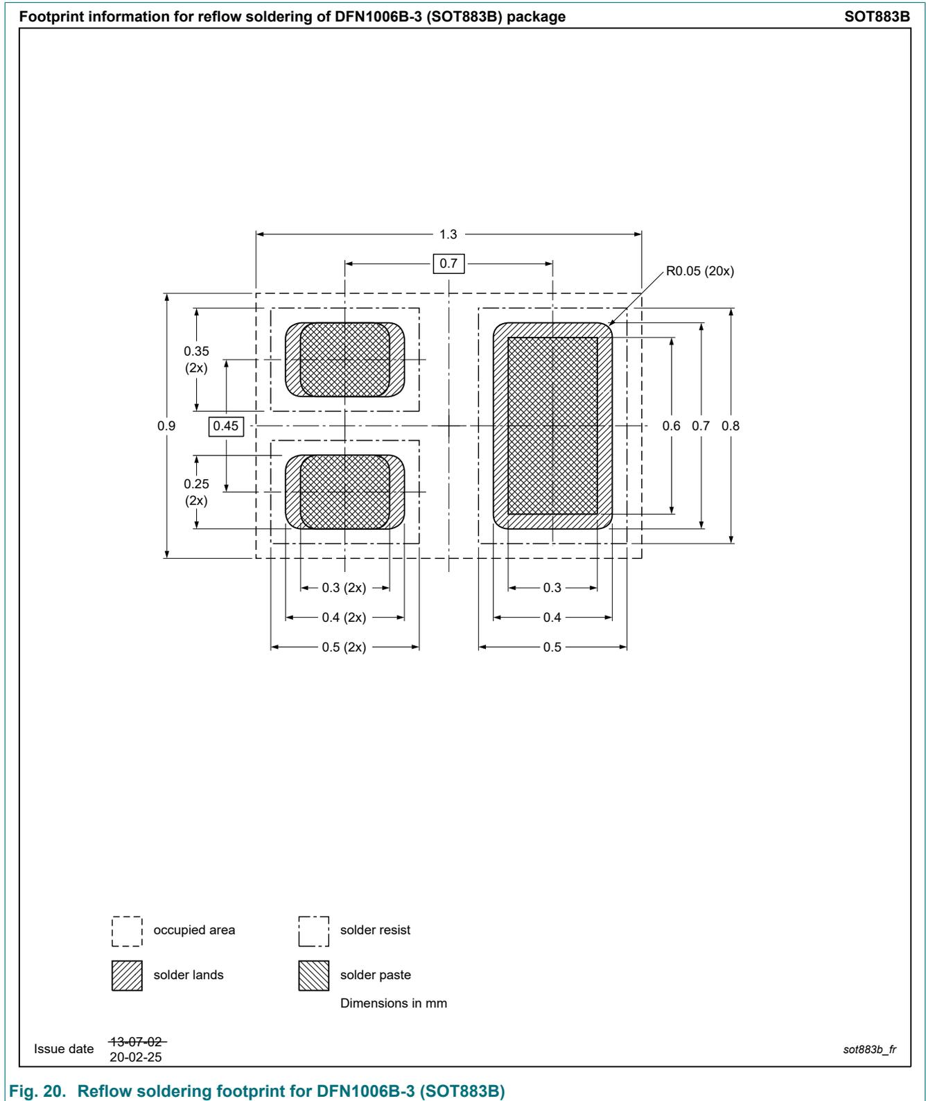
Fig. 20. Reflow soldering footprint for DFN1006B-3 (SOT883B)
