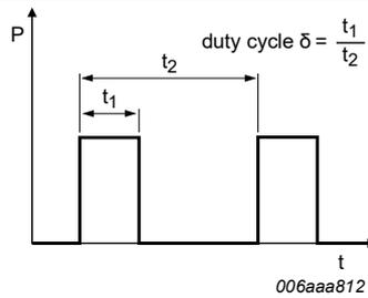
Fig. 18. Duty cycle definition
