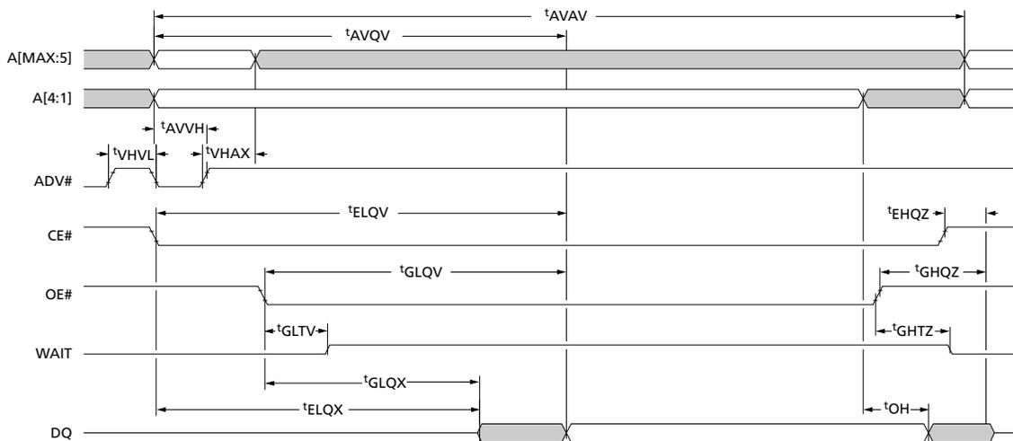
Note: 1. WAIT shown deasserted during asynchronous read mode (RCR10 = 0, WAIT asserted LOW).
