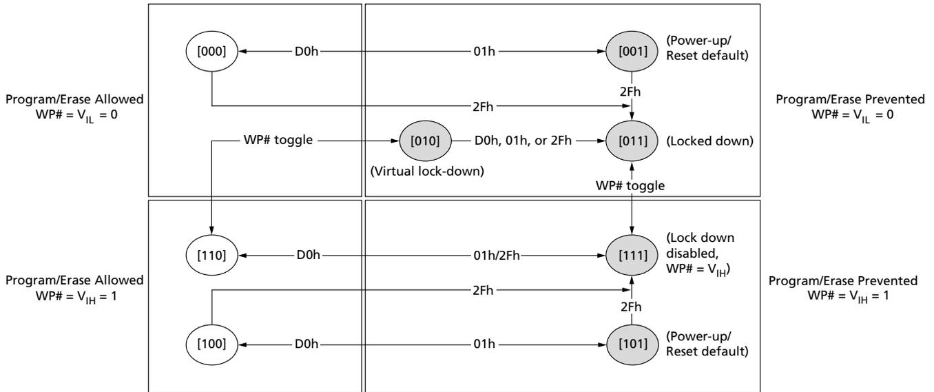
Note: 1. D0h = UNLOCK command; 01h = LOCK command; 60h (not shown) LOCK SETUP command; 2Fh = LOCK DOWN command.
