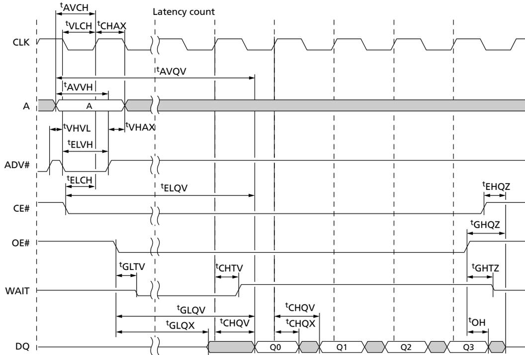
Note: 1. WAIT is driven per OE# assertion during synchronous array or nonarray read. WAIT asserted during initial latency and deasserted during valid data (RCR10 = 0, WAIT asserted LOW).
