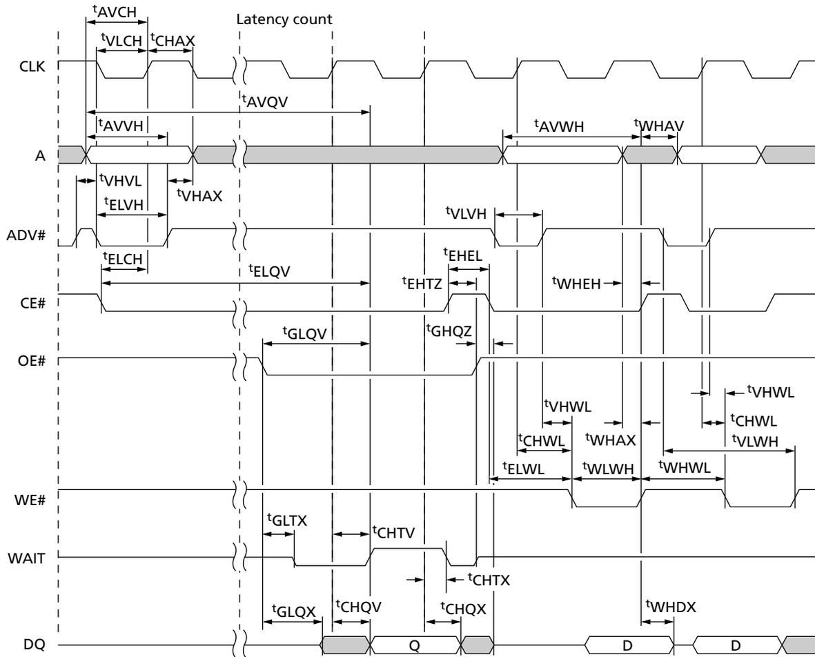
Note: 1. WAIT shown de-asserted and High-Z per OE# de-assertion during WRITE operation (RCR10 = 0, WAIT asserted LOW). Clock is ignored during WRITE operation.
