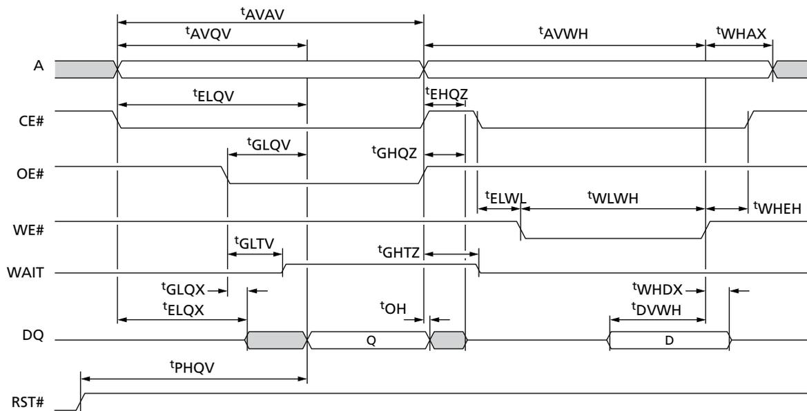
Note: 1. WAIT de-asserted during asynchronous read and during write. WAIT High-Z during write per OE# deasserted.
