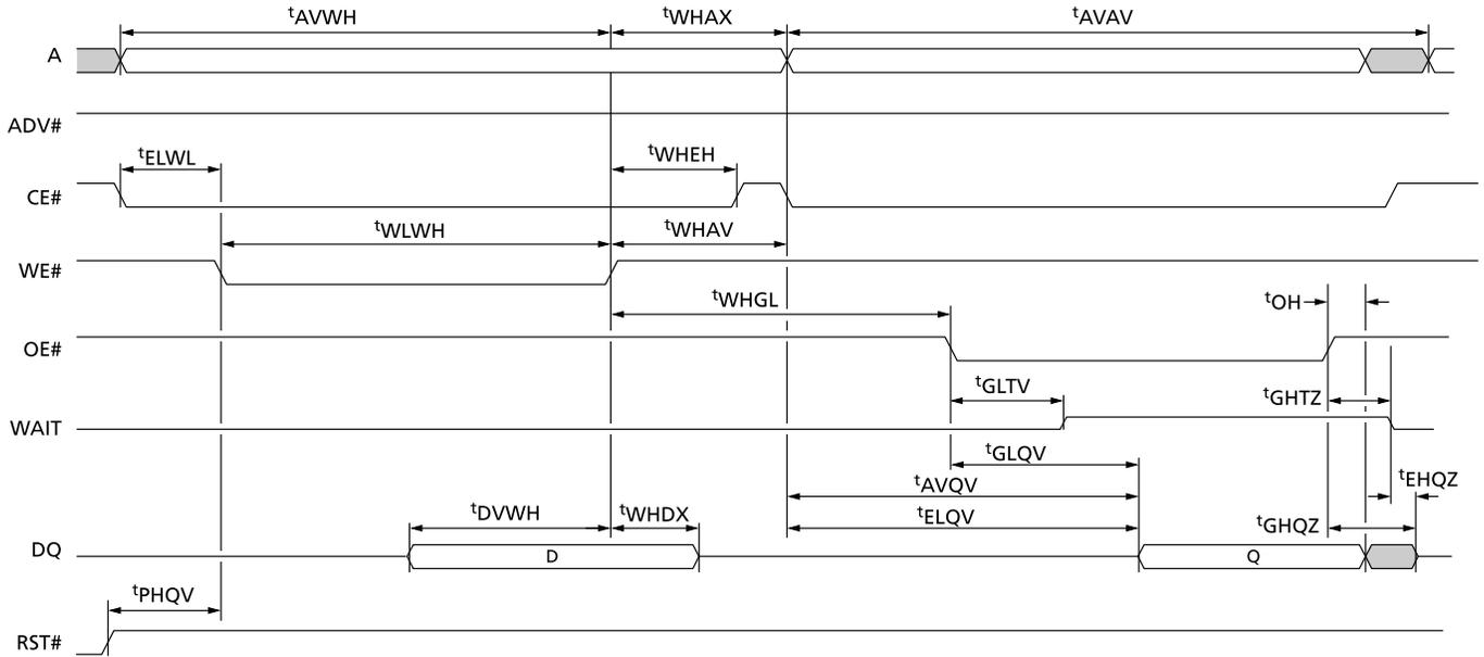
Figure 35: Synchronous Read to Write Timing
