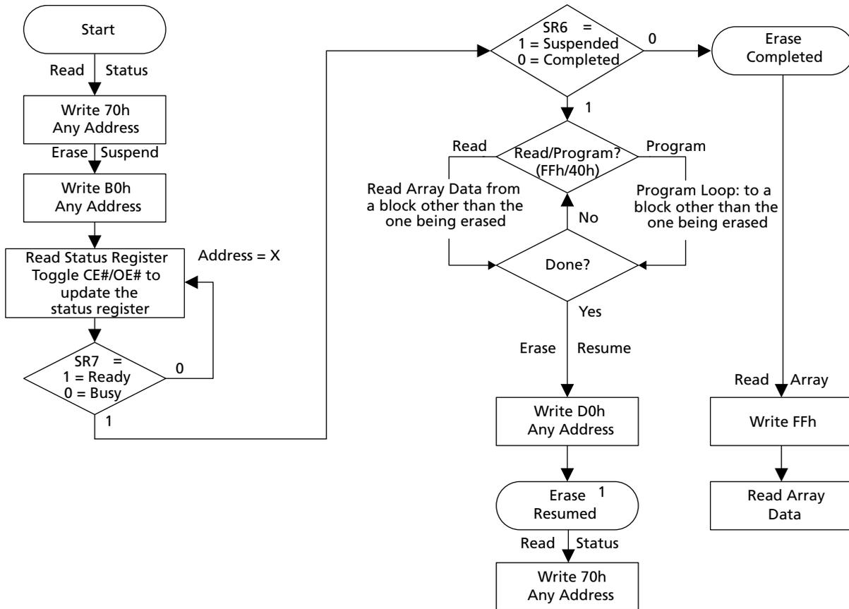
Note: 1. The  $t_{ERS/SUSP}$  timing between the initial BLOCK ERASE or ERASE RESUME command and a subsequent ERASE SUSPEND command should be followed.
