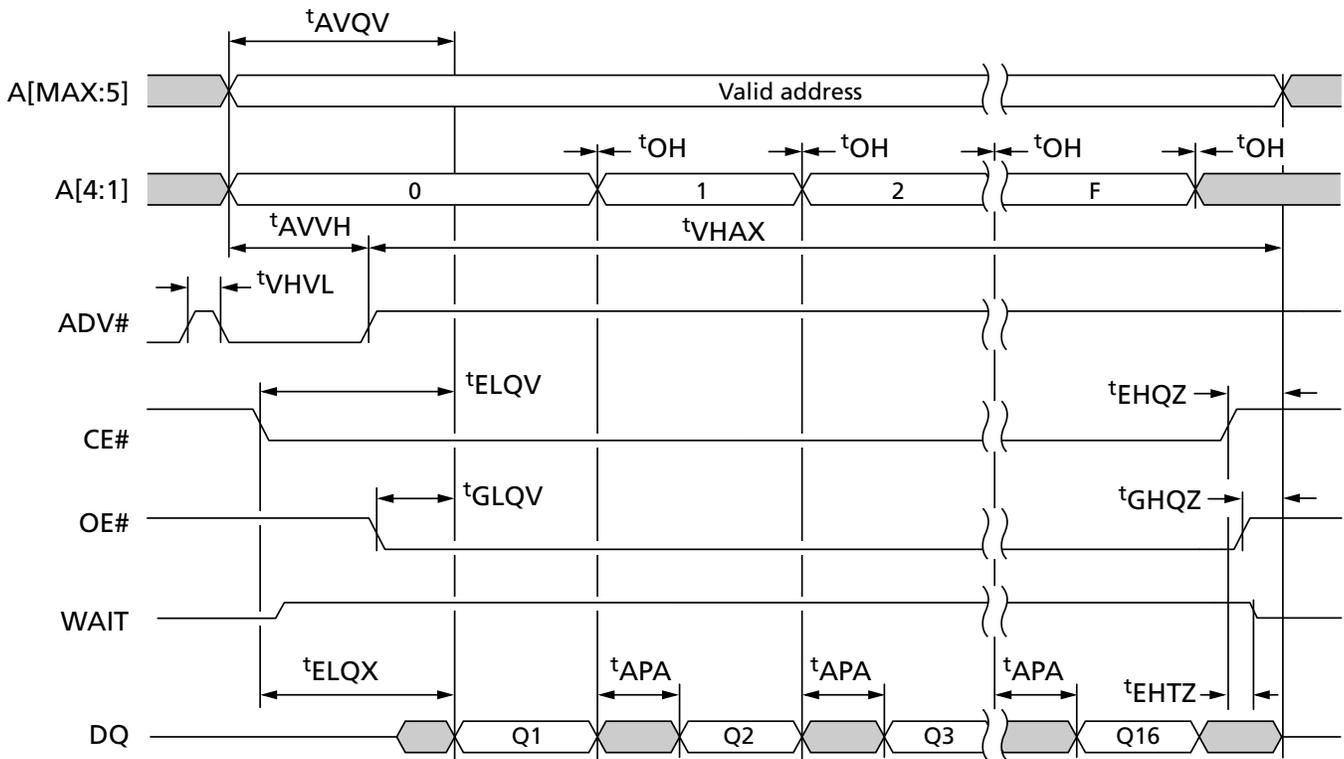
Note: 1. WAIT shown deasserted during asynchronous read mode (RCR10 = 0, WAIT asserted LOW).
