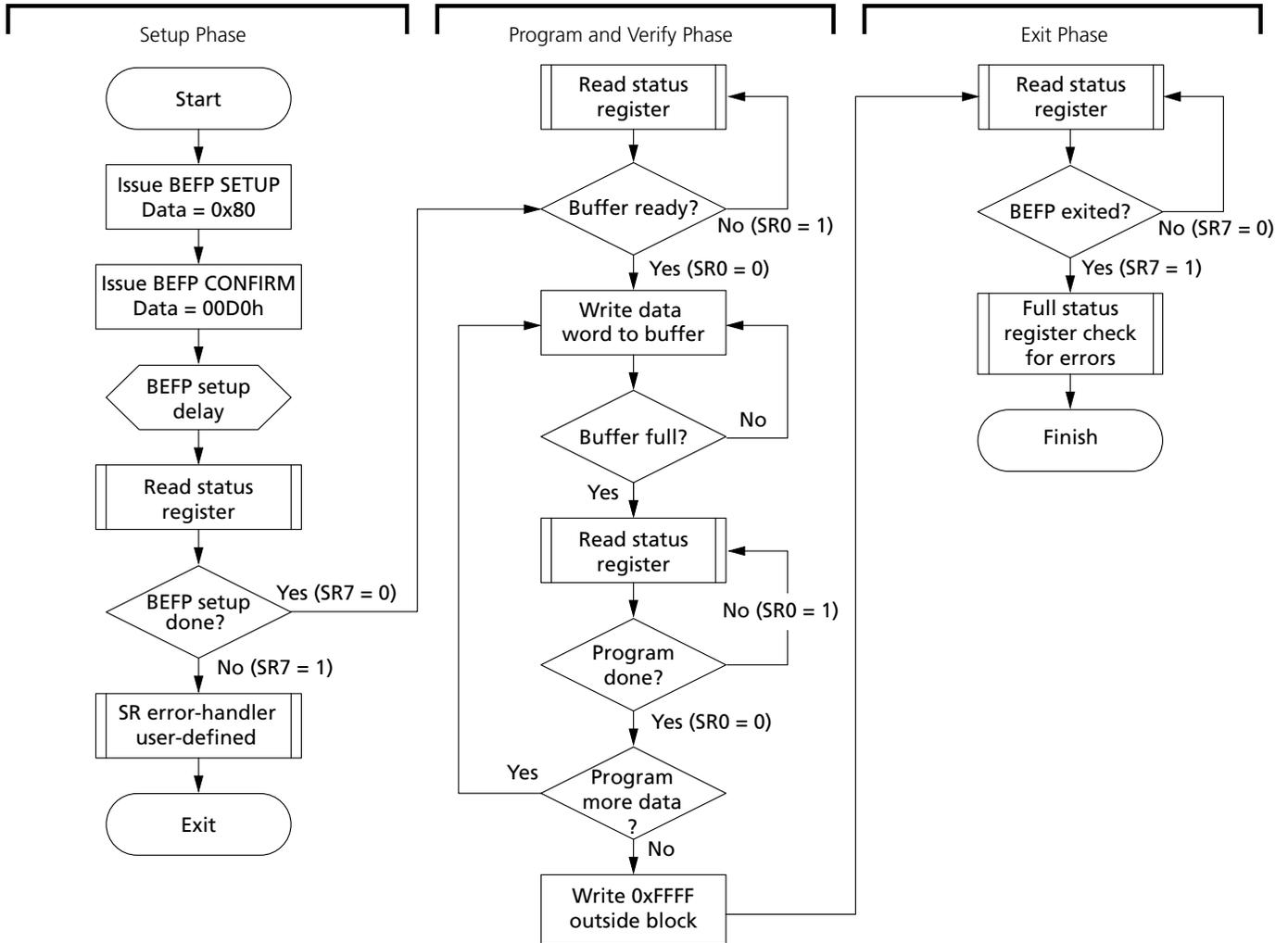
Figure 16: Block Erase Procedure
