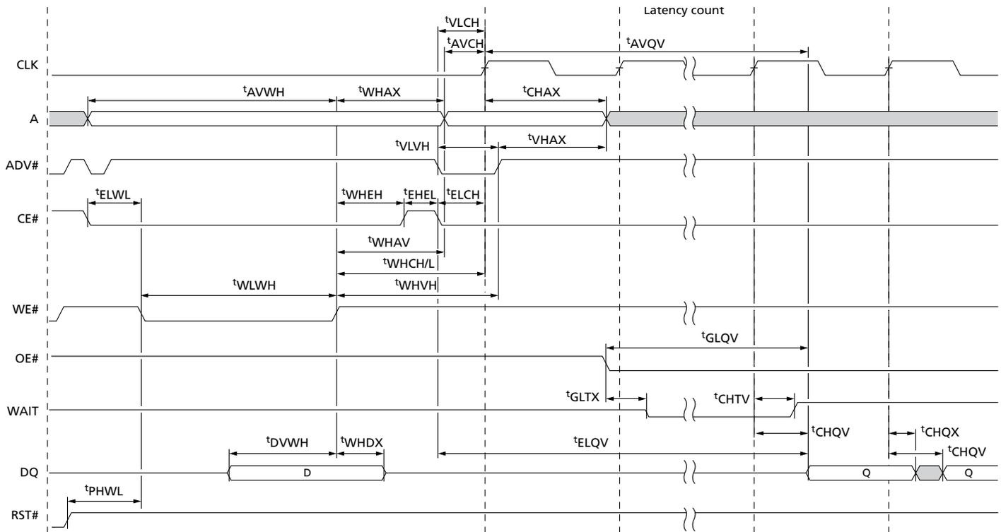
Note: 1. WAIT shown de-asserted and High-Z per OE# de-assertion during WRITE operation (RCR10 = 0, WAIT asserted LOW).
