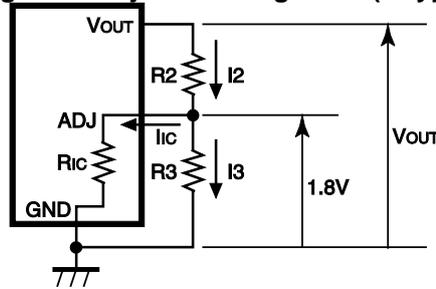
The Output Voltage of Regulator in R1130xxxxC may be adjustable for any output voltage between its 1.8V reference and its V<sub>DD</sub> setting level. An external pair of resistors is required, as shown in Figure 1.
