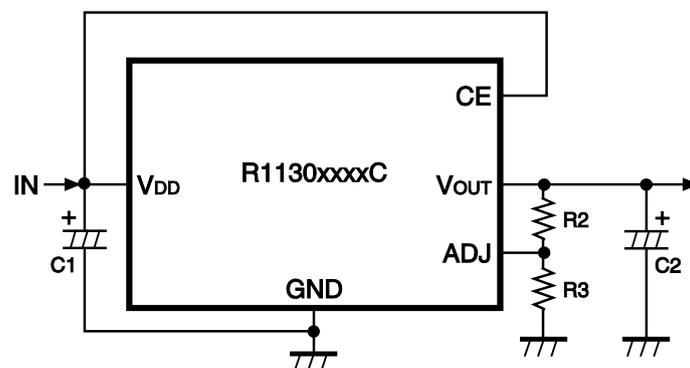
$C1=C2=0.1\mu\text{F}$ , R2, R3: Refer to the Technical Notes on Output Voltage setting of C type.
