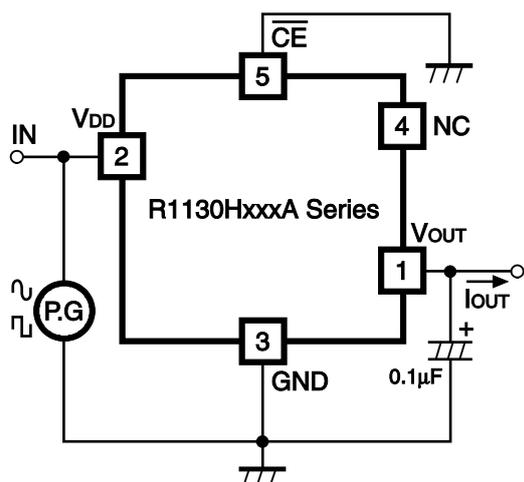
Fig.3 Ripple Rejection, Line Transient Response Test Circuit
