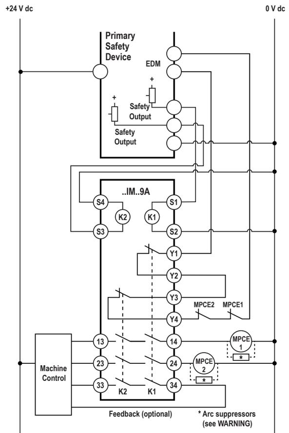
These wiring diagrams are labeled ..IM..9A. The wiring for model ..IM..11A is similar, but not identical because of the different contact arrangement.
