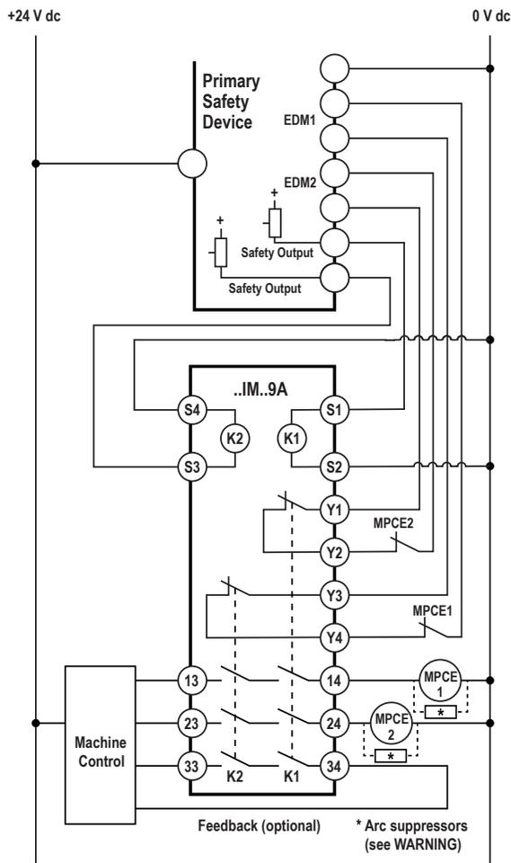
Figure 6. Generalized wiring to a 2-channel primary safety device with two current-sourcing safety outputs and one monitoring input.
