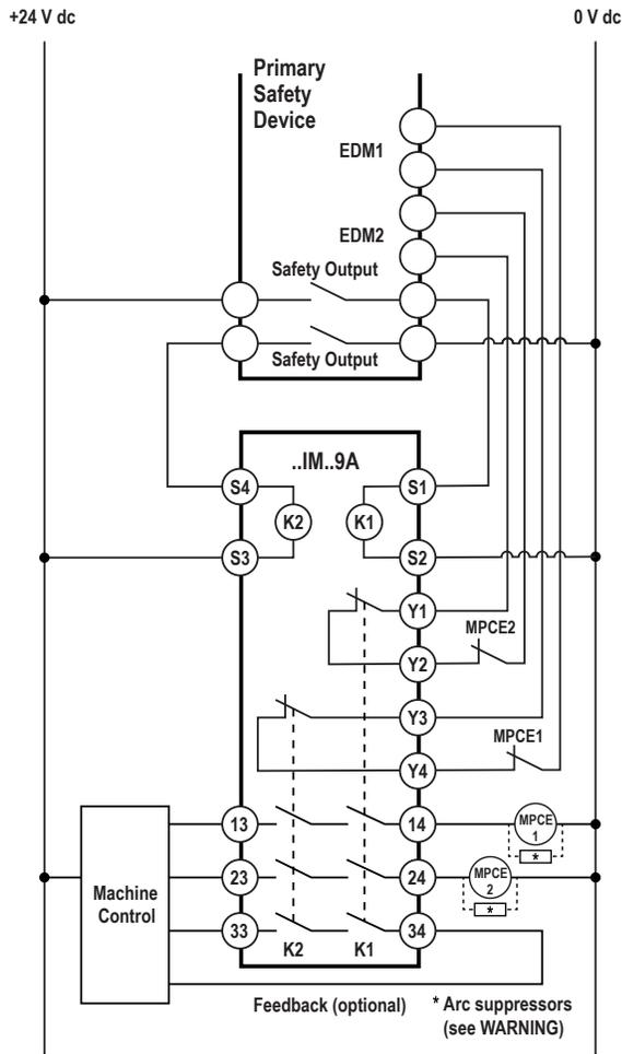
Figure 4. Generalized wiring to a 2-channel primary safety device with two hard-contact safety outputs and one monitoring contact feedback input.
