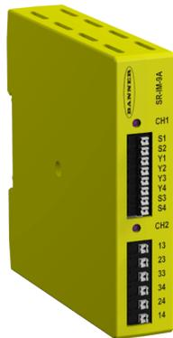
The SR-IM-9A and SR-IM-11A Interface Module provides isolated safety output contacts for a primary safety device (for example, a safety light screen or safety module) with solid-state or hard contact outputs and external device monitoring (EDM) capability.
