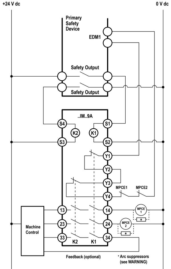
These wiring diagrams are labeled ..IM..9A. The wiring for model ..IM..11A is similar, but not identical because of the different contact arrangement.
