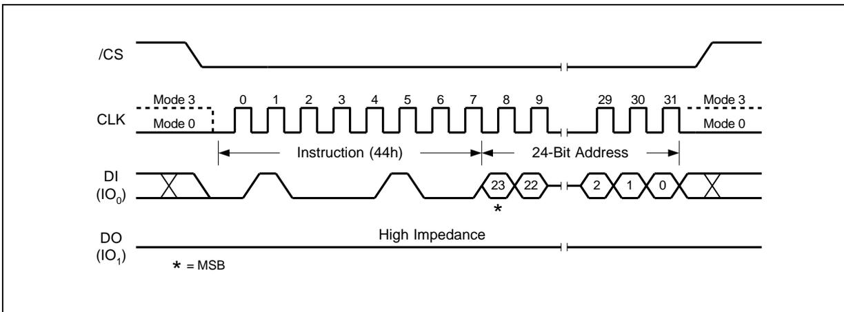
Figure 44. Erase Security Registers Instruction (SPI Mode only)
