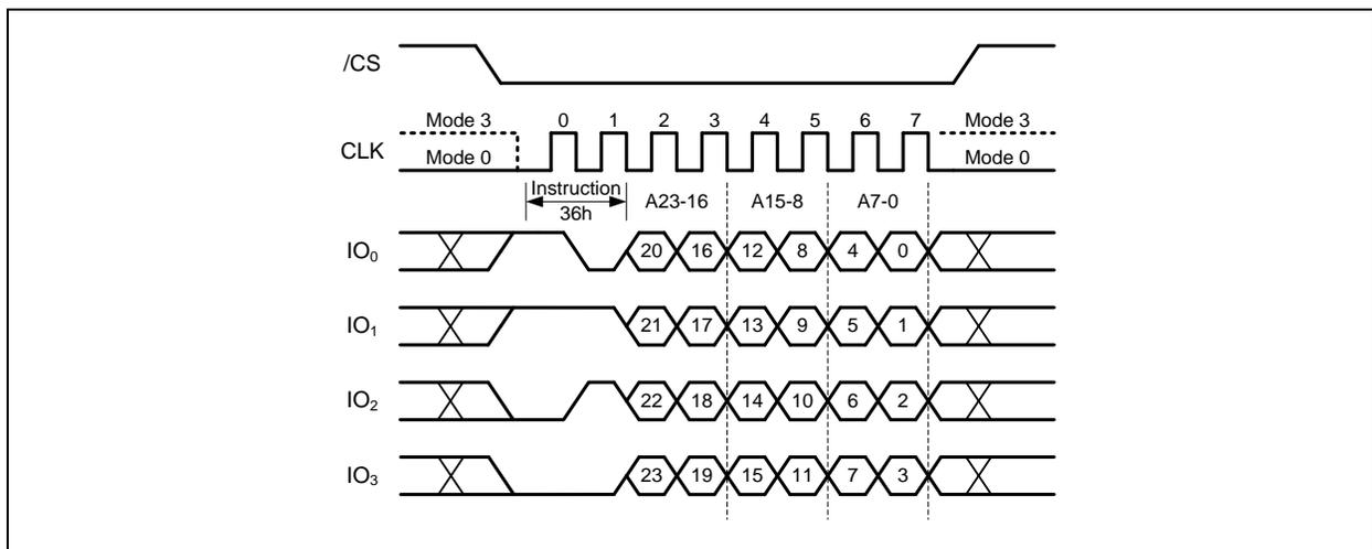
Figure 51b. Individual Block/Sector Lock Instruction (QPI Mode)
