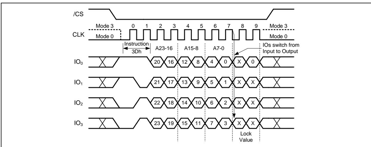
Figure 53b. Read Block Lock Instruction (QPI Mode)
