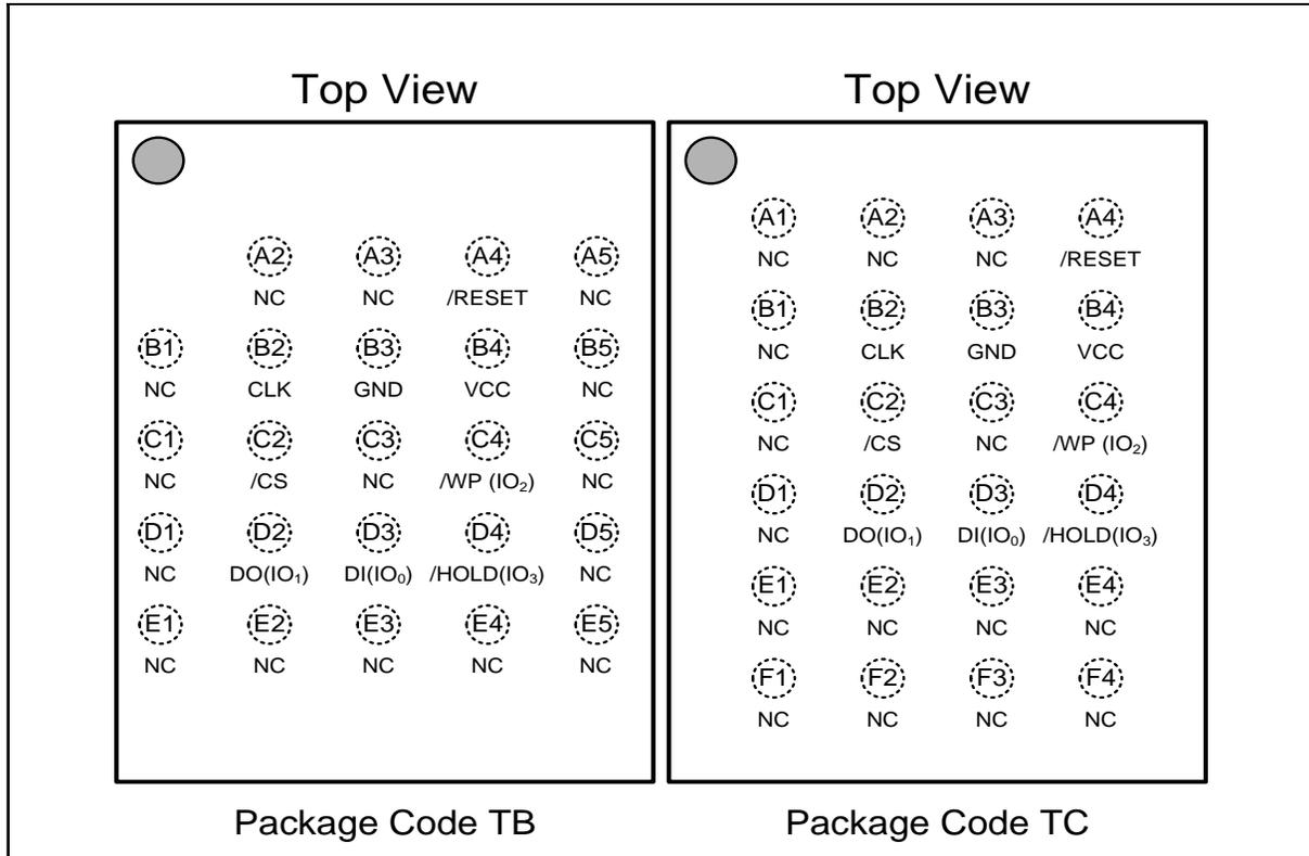
Figure 1d. W25Q32FW Ball Assignments, 24-ball TFBGA 8x6-mm (Package Code TB, TC)
