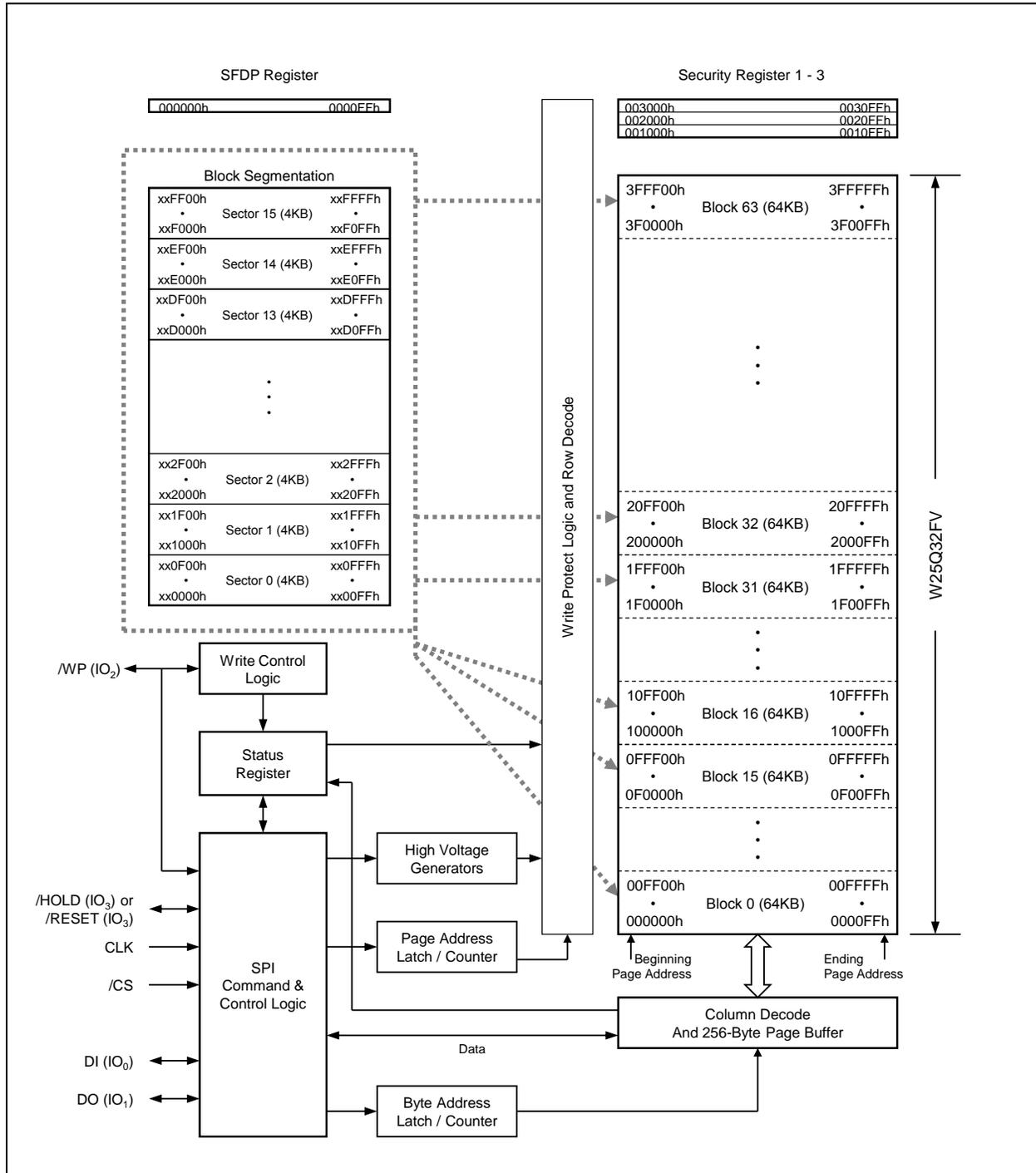
Figure 2. W25Q32FW Serial Flash Memory Block Diagram
