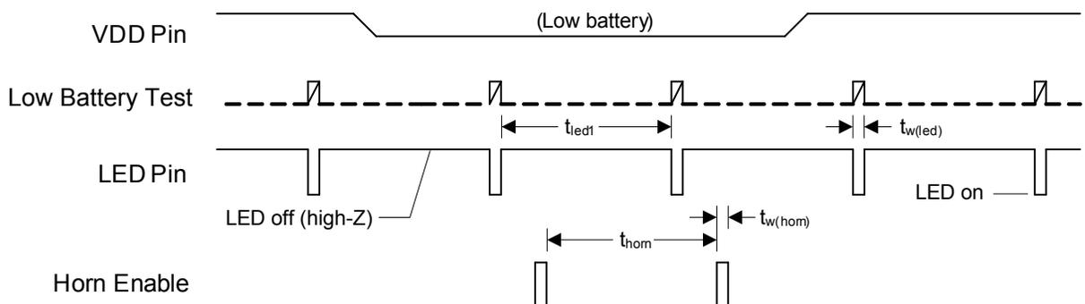
**Local Smoke Detection/Test Alarm Condition**
