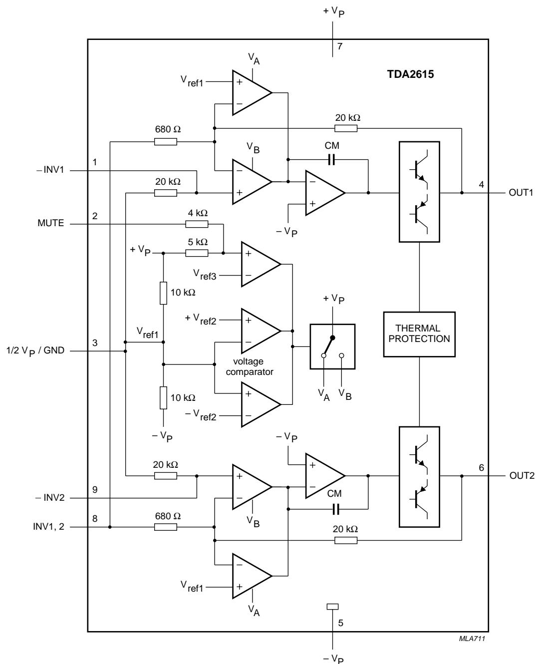
Fig.1 Block diagram.
