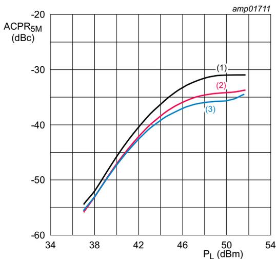
$V_{DS} = 32\text{ V}; I_{Dq} = 1450\text{ mA}; V_{GS(amp)peak} = 1.1\text{ V}.$
