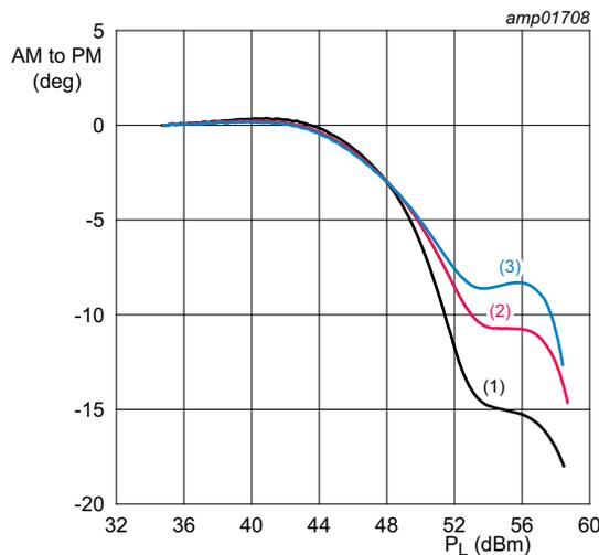
$V_{DS} = 32\text{ V}$ ;  $I_{Dq} = 1450\text{ mA}$ ;  $V_{GS(amp)peak} = 1.1\text{ V}$ ;  $t_p = 100\text{ }\mu\text{s}$ ;  $\delta = 10\text{ }\%$ .
