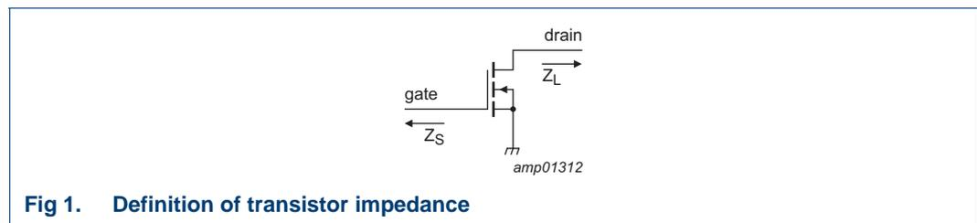
**Fig 1. Definition of transistor impedance**
