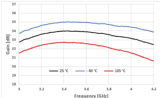
**Figure 9. Gain Flatness @ VDD = 5.0V**
