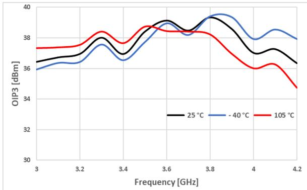
**Figure 24. OIP3 @ VDD = 3.3V**
