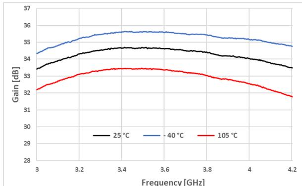
**Figure 8. Gain Flatness @ VDD = 3.3V**
