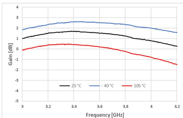
**Figure 10. Gain Flatness @ VDD = 3.3V**
