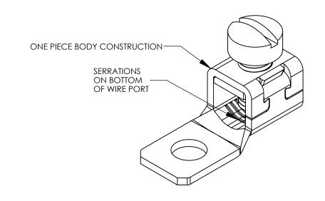
\* MULTIPLE WIRES MUST BE TWISTED TOGETHER BEFORE INSERTION INTO CONNECTOR
