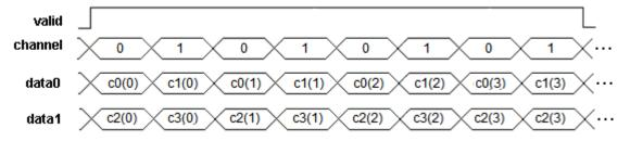
The channel signal remains a single wire, not a wire for each data wire. It counts over 0 to ChanCycleCount -1.
