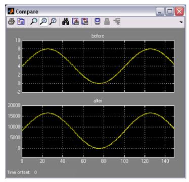
For example, a **Mult** block with both input data types specified as **sfix16\_En15** naturally has an output type of **sfix32\_En30**. The specified output data type has two fewer fractional bits than the natural input data type. Therefore, if you specify the output data type as **sfix32\_En28**, the output numerical value is effectively multiplied by four, and a 1\*1 input gives an output value of 4.
