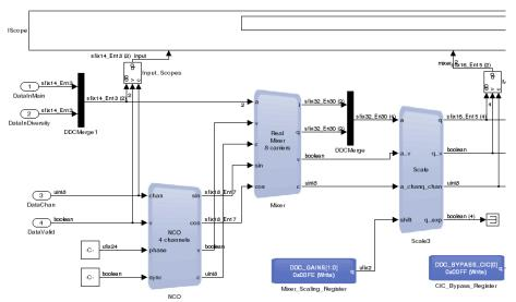
Note: The inputs, NCO, and mixer stages show with Simulink signal formats turned on.
