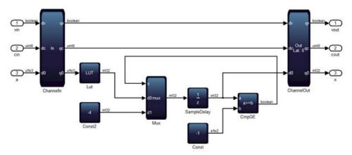
DSP Builder relocates the sample delay, to save registers, to the Boolean signal that drives the s-input of the 2-to-1 **Mux** block. You may see a mismatch in the first cycle and beyond, depending on the contents of the LUT.
