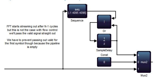
The latency that the **ChannelOut** block reports is therefore not 4096 + the automatic pipelining value, but just the pipelining value.
