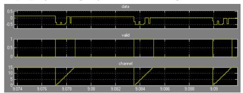
The number of input integrator sections is 4, and the number of output comb sections is 1. The lower data rate reduces the size of the overall group of 4 CICs. The Help page also reports the gain for the DCIC to be 1,048,576 or approximately 2^20. The Help page also shows how DSP Builder combines the four channels of input data on a single output data channel. The comb section utilization (from the DSP Builder menu) confirms the 25% calculation for the folding factor.
