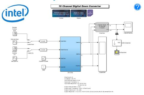
The top-level testbench includes **Control** and **Signals** blocks, and some Simulink blocks to generate source signals and visualize the output. The full power of the Simulink blocksets is available for your design.
