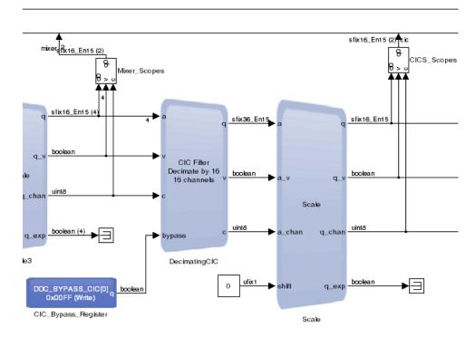
Two main blocks exist—the **DecimatingCIC** and the **Scale** block. To configure the CIC Filter, double click on the **DecimatingCIC** block.
