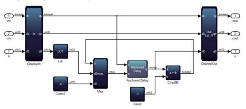
To make a control unit design resistant to automated delay redistribution and to solve most hardware FSM designs that fail to match simulation, replace every **SampleDelay** block with the **Anchored Delay** block from the **Control** folder in the Additional libraries. When the valid-in first goes high, the **Anchored Delay** block outputs one (or more) zeros, otherwise it behaves just like an ordinary **SampleDelay** block.
