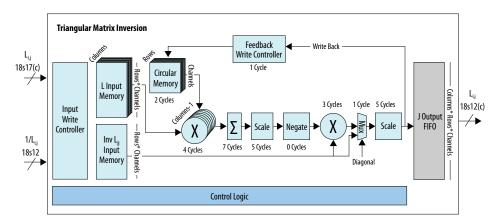
This design supports single-precision floating-point Cholesky matrix inversion. DSP Builder requires a single-precision floating-point input for the floating point inversion.
