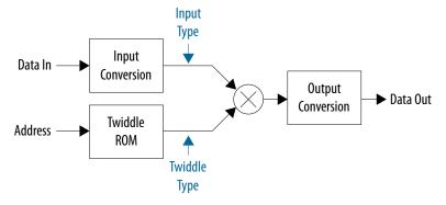
An FFT with 2N points has N radix-2 stages and (conceptually) N-1 twiddle multipliers. In practice, DSP Builder optimizes away many of the twiddle multipliers. However, they still need entries in the twiddle specification.
