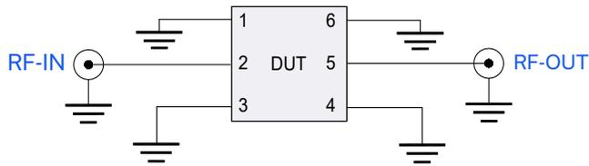
Fig 1. Block diagram of Test Circuit used for characterization, Test board TB-934-1C+ Conditions: Attenuation, VSWR: Pin=0 dBm
