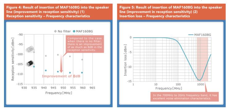
Thus, it can be seen that the application of MAF1608G to audio lines is extremely effective as a solution to the problem of degradation of reception sensitivity in smartphones. But what about the problem of voice distortion caused by insertion?
