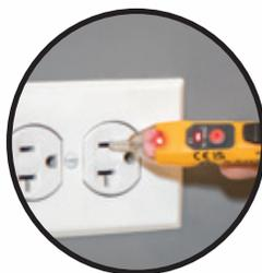
When voltage is detected, a high intensity, bright red LED illuminates and an audible tone will sound
