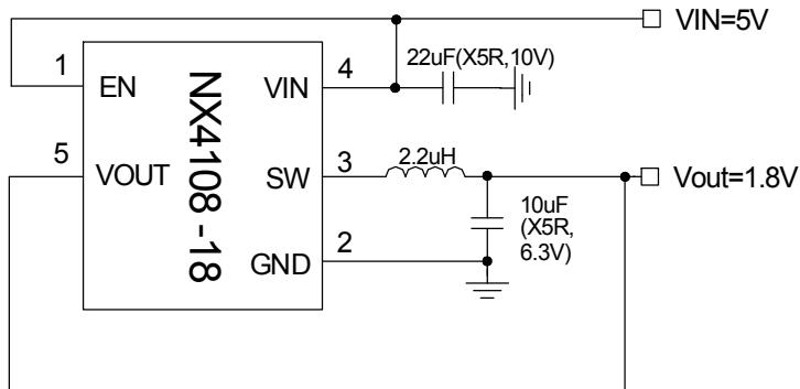
Figure1 -Typical application of NX4108-18
