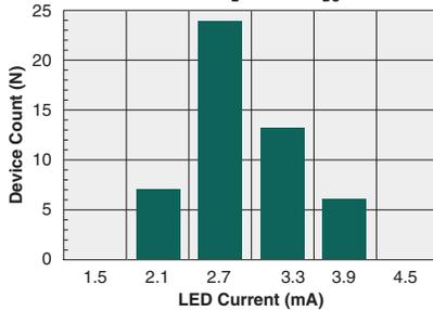
Typical I<sub>F</sub> for Switch Dropout
