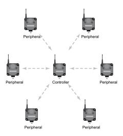
Figure 4: Star network in broadcast mode configuration
