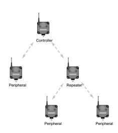
Figure 5: Tree network in broadcast mode configuration
