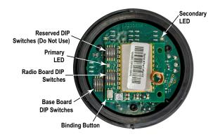
Figure 1: Binding button, LEDs, and DIP switches
