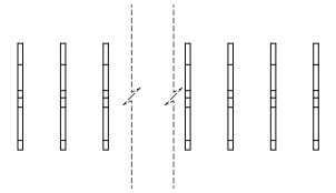
NOTE: **CONTACTS ARE HELD IN** A CARRIER FOR EASE OF ASSEMBLY
