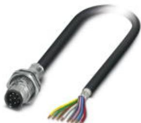
Flush-type plug, shielded, 8-pos., M12, A-coded, rear/screw mounting with M16 thread, with 1 m cable, 8 x 0.25 mm<sup>2</sup>
