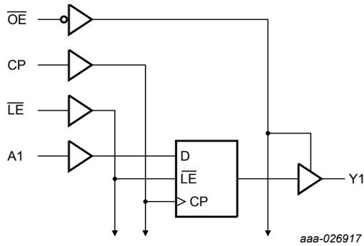
Fig. 1. Logic diagram
