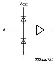
Fig. 3. Typical input (data or control)
