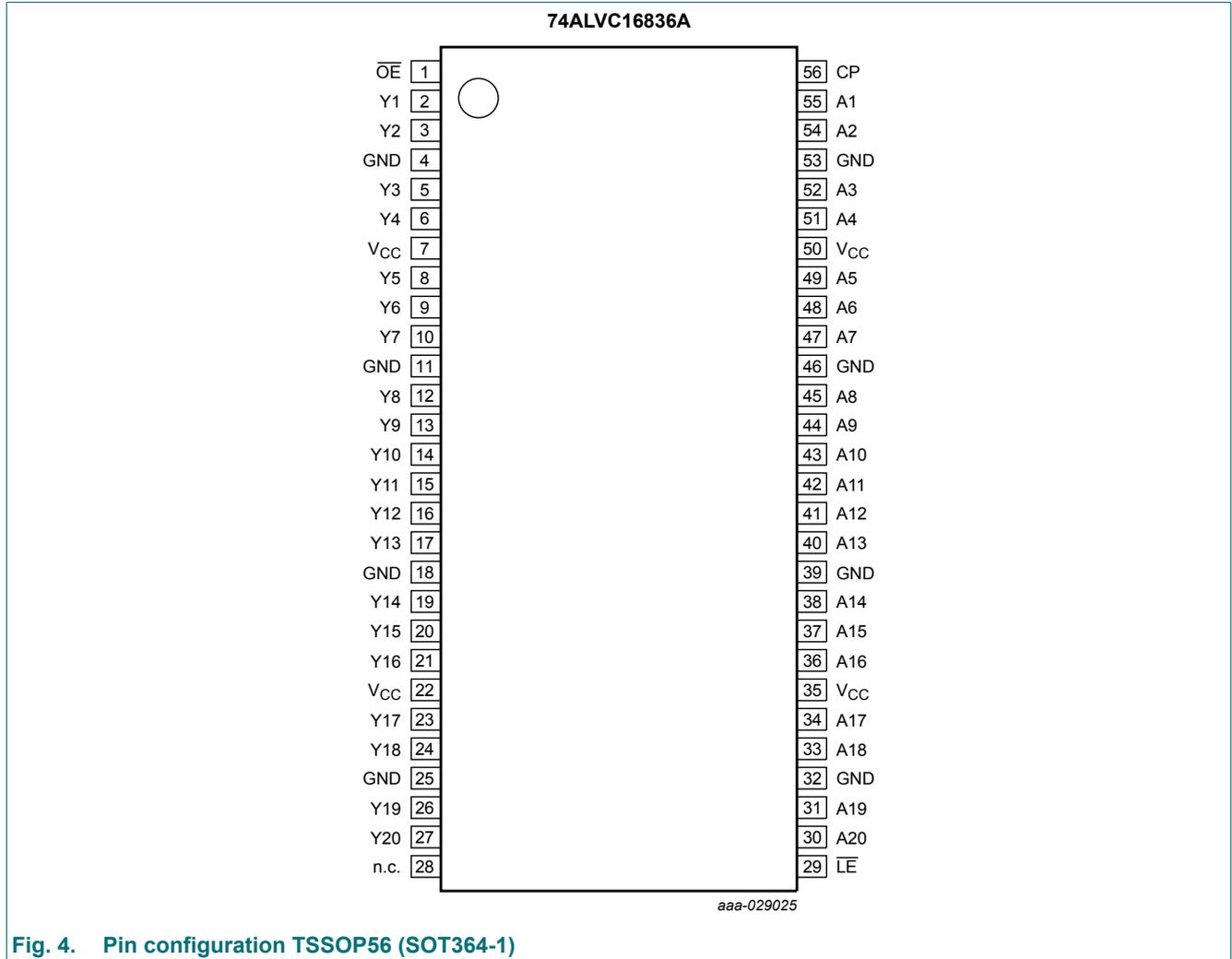
Fig. 4. Pin configuration TSSOP56 (SOT364-1)
