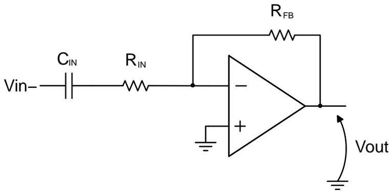
$$A_v = \frac{V_{out}}{V_{in-}} = -\frac{R_{FB}}{R_{IN}} \quad (\text{eq. 10})$$
