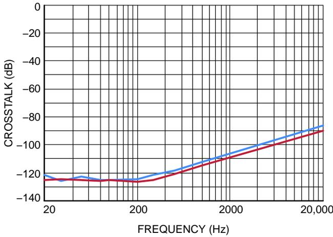
**Figure 11. Crosstalk vs. Frequency,**
