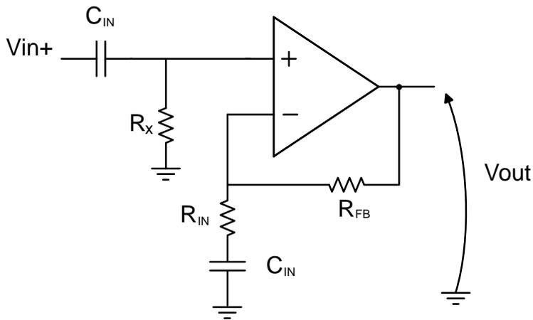
$$A_v = \frac{V_{out}}{V_{in+}} = 1 + \frac{R_{FB}}{R_{IN}} \quad (\text{eq. 11})$$
