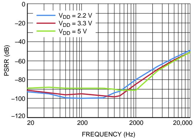
**Figure 14. Power Supply Rejection Ratio vs.**
