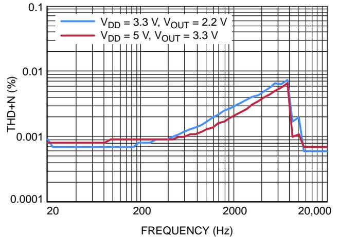
Figure 8. THD+N vs. Frequency,  $R_L = 600\ \Omega$
