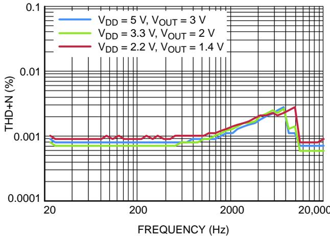
Figure 7. THD+N vs. Frequency,  $R_L = 2.5\text{ k}\Omega$
