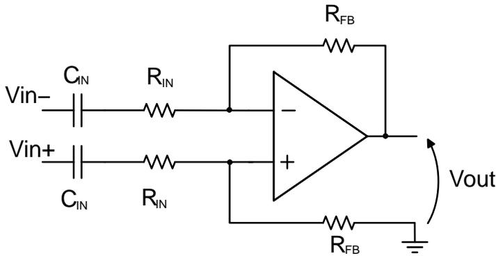
$$A_v = \frac{V_{out}}{V_{in+} - V_{in-}} = \frac{R_{FB}}{R_{in}} \quad (\text{eq. 9})$$
