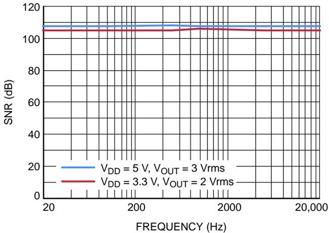
**Figure 13. Signal-to-Noise Ratio vs.**
