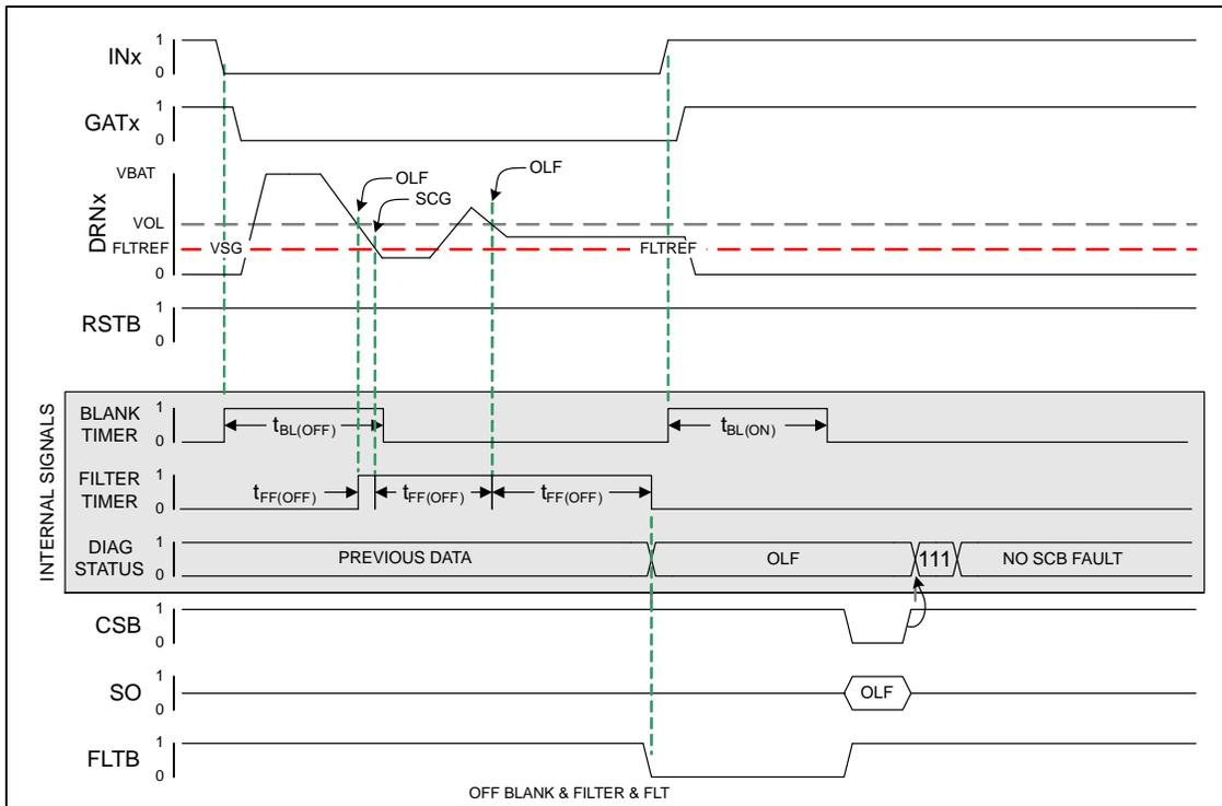
**Figure 31. Filter Timer Started When Falling Through OLF Threshold During Blank Timer, Re-started When Falling Through SCG Threshold, Re-started When Falling Through OLF Threshold – OFF-State Diagnostic Status Acquisition Time Extended by Filter Timer**
