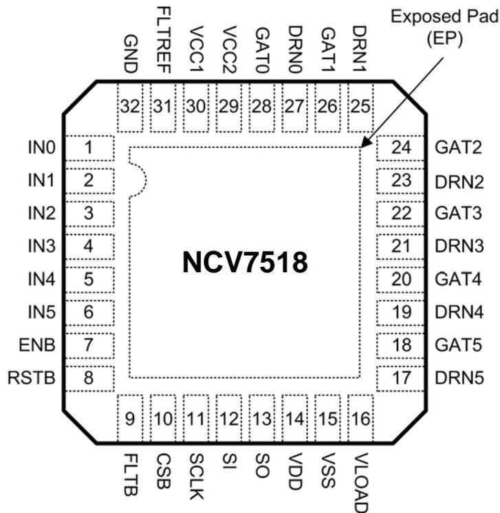
Figure 3. 32 Pin QFN Exposed Pad Pinout (Top View)
