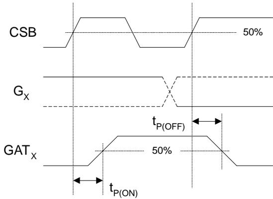
Figure 5. Gate Driver Timing Diagram – Serial Input
