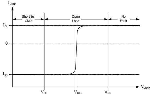
**Figure 13. DRN<sub>X</sub> Bias and Fault Detection Zones**
