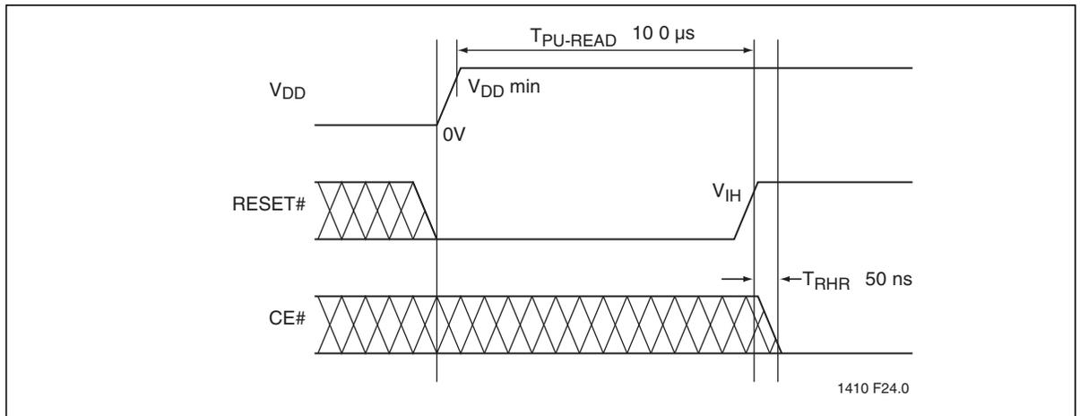
**Figure 4:** Power-Up Diagram
