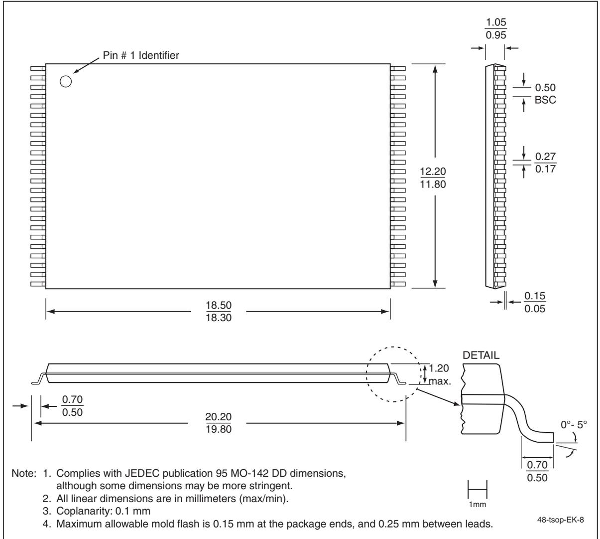
**Figure 26:** 48-lead Thin Small Outline Package (TSOP) 12mm x 20mm,
