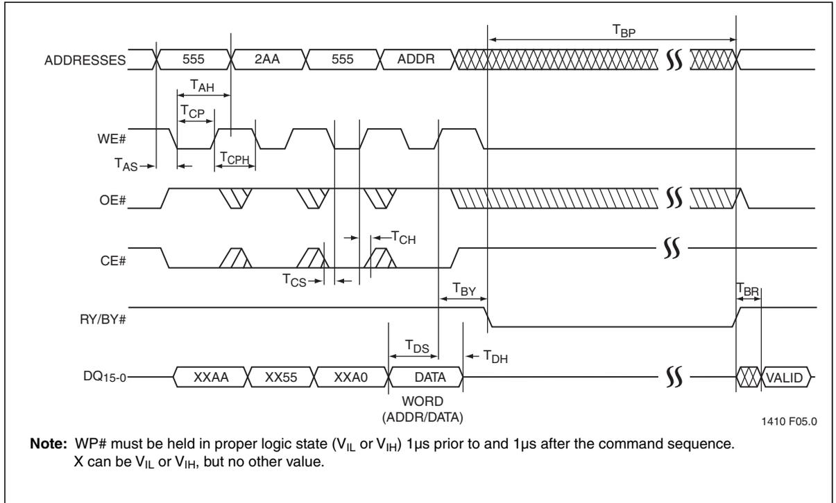
**Figure 7:** CE# Controlled Program Cycle Timing Diagram
