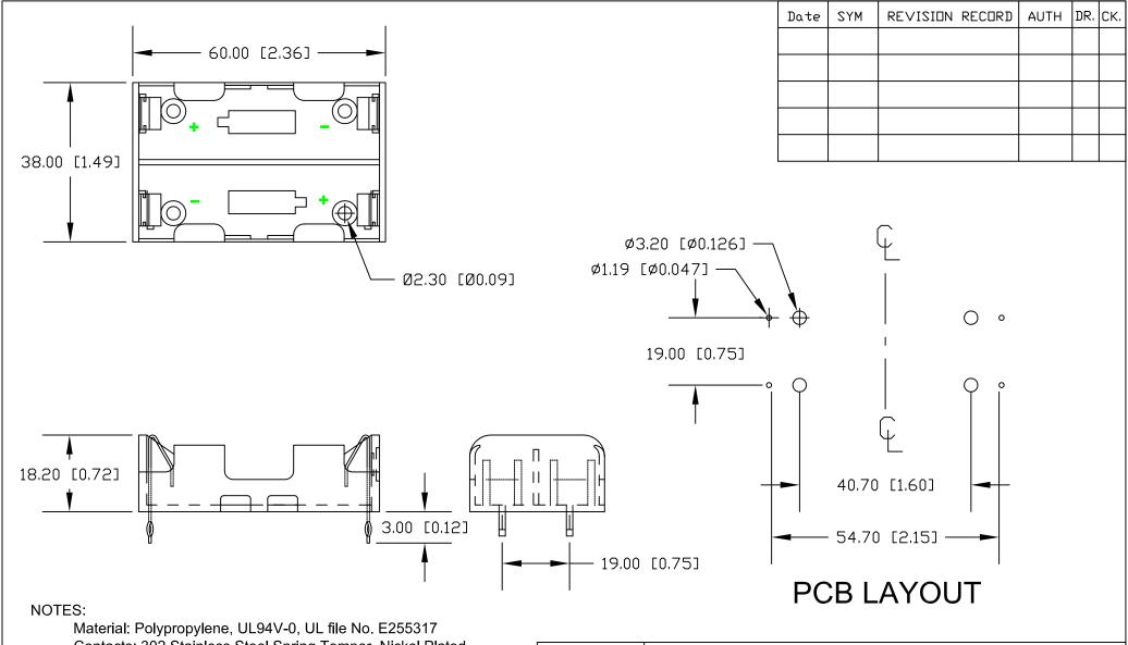
Contacts: 302 Stainless Steel Spring Temper, Nickel Plated
