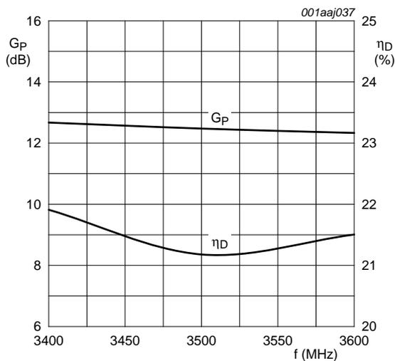
$V_{DS} = 28\text{ V}$ ;  $I_{Dq} = 1050\text{ mA}$ ; Single Carrier IS-95; PAR = 9.7 dB at 0.01 % probability.
