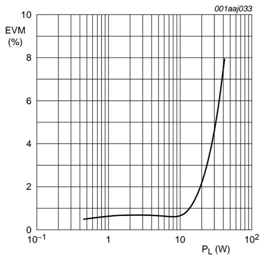
$V_{DS} = 28$  V;  $I_{Dq} = 1050$  mA;  $f = 3500$  MHz.
