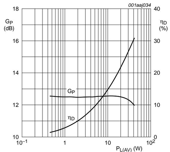
$V_{DS} = 28$  V;  $I_{Dq} = 1050$  mA;  $f = 3500$  MHz.
