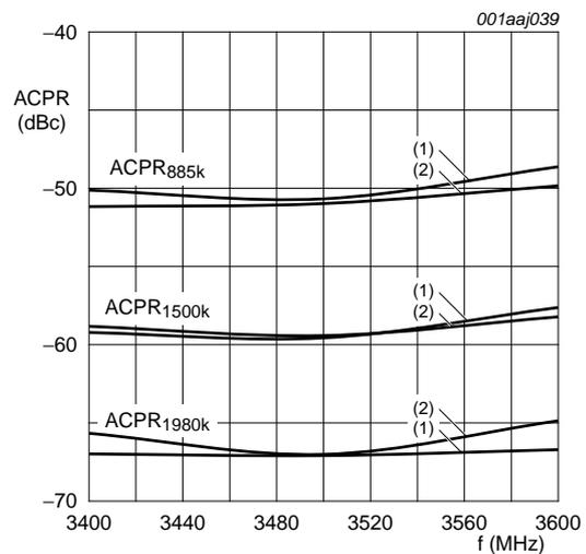
$V_{DS} = 28\text{ V}$ ;  $I_{Dq} = 1050\text{ mA}$ ; single carrier IS-95; PAR = 9.7 dB at 0.01 % probability.
