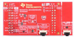
Figure 1-1. BOOSTXL-BASSENSORS Plug-in Module
