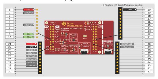
Figure 2-2. BoosterPack™ Plug-In Module Pinout
