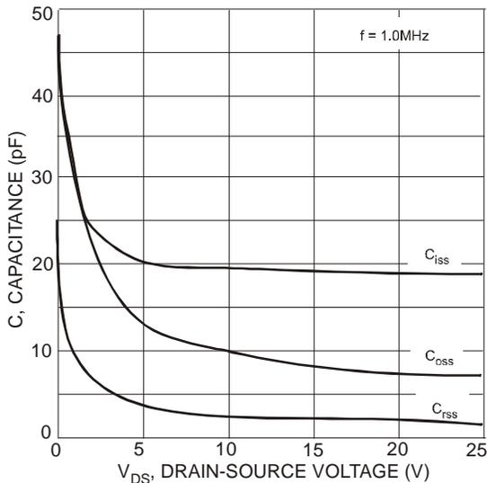
Fig. 5 Typical Capacitance
