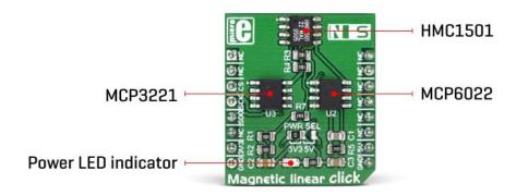
The HMC1501 IC is targeted towards working with both bipolar and unipolar single-ended inputs. Each input is labeled as S1 to S8. When a specific channel is selected by using the A0 to A2 pins, it will be switched to the output pin, labeled as D. For the improved stability, each pin is equipped with the 100nF parallel capacitor and  $100\Omega$  series resistance. The input and the output signal pins are routed to the standard 2.54mm pitch 2x5 pins header on the Click board<sup>TM</sup>.
