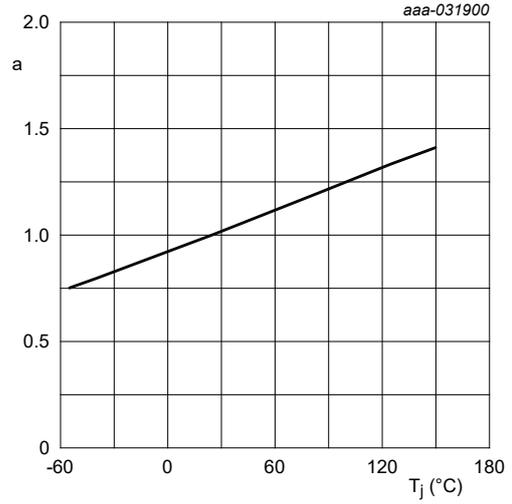
$$a = \frac{R_{DSon}}{R_{DSon}(25^\circ\text{C})}$$
