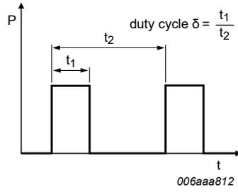
Fig. 17. Duty cycle definition
