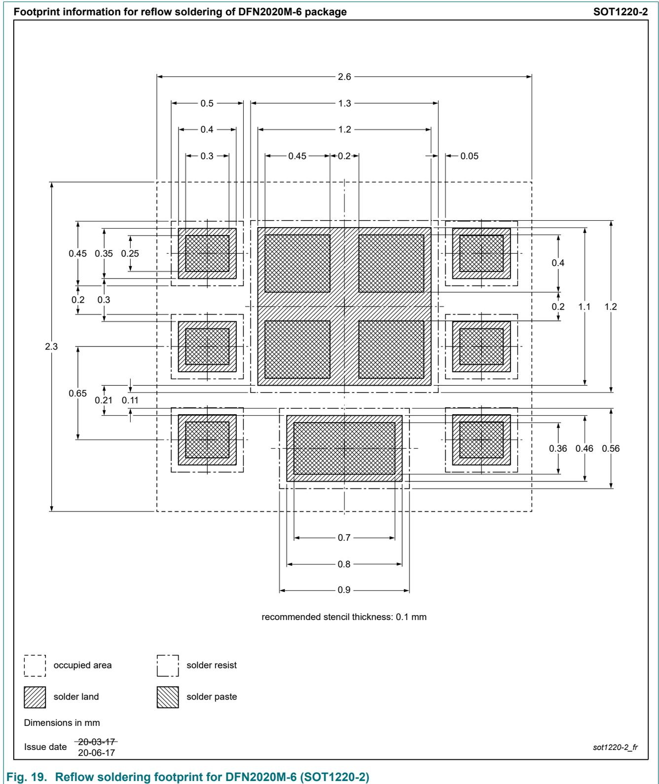
**Fig. 19. Reflow soldering footprint for DFN2020M-6 (SOT1220-2)**
