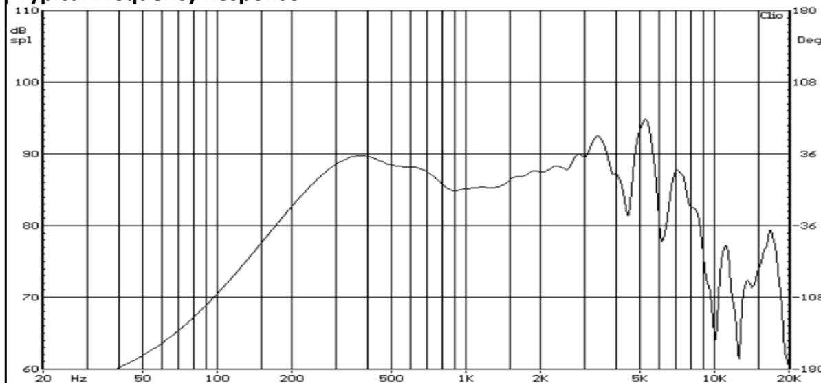
Measured on axis at a distance of 1m with 1W input power
