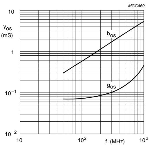
$V_{DS} = 8$  V;  $V_{G2-S} = 4$  V;  $I_D = 10$  mA;  $T_{amb} = 25$  °C.
