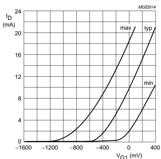
$V_{D-S} = 8$  V;  $V_{G2-S} = 4$  V;  $T_{amb} = 25$  °C.
