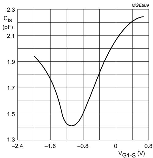
$V_{DS} = 8\text{ V}; V_{G2-S} = 4\text{ V}; f = 1\text{ MHz}; T_{amb} = 25\text{ }^{\circ}\text{C}.$
