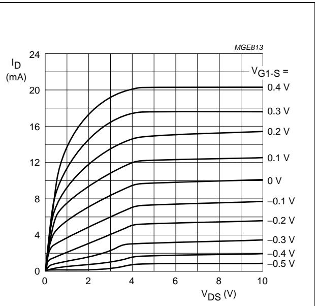
$V_{G2-S} = 4$  V;  $T_{amb} = 25$  °C.
