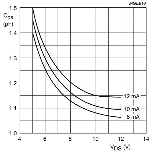
$V_{G2-S} = 4\text{ V}; f = 1\text{ MHz}; T_{amb} = 25\text{ }^{\circ}\text{C}.$
