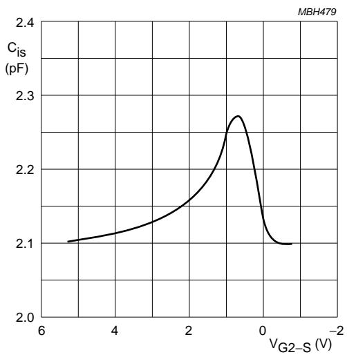
$V_{DS} = 8\text{ V}; V_{G1-S} = 0\text{ V}; f = 1\text{ MHz}; T_{amb} = 25\text{ }^{\circ}\text{C}.$
