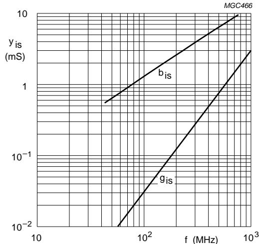
$V_{DS} = 8$  V;  $V_{G2-S} = 4$  V;  $I_D = 10$  mA;  $T_{amb} = 25$  °C.
