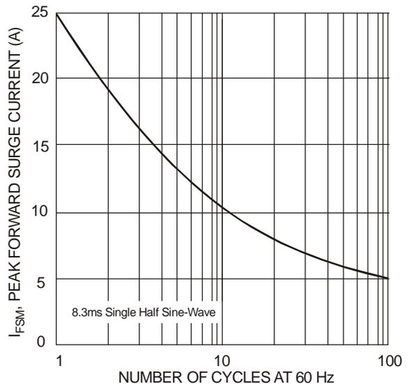
Fig. 6 Maximum Non-Repitative Peak Forward Surge Current
