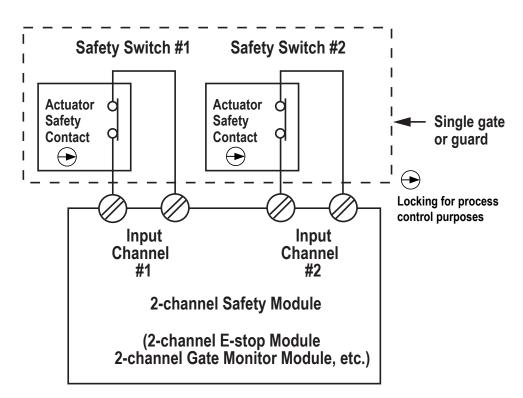
Figure 10. Actuator safety contacts (circle with arrow symbol)
