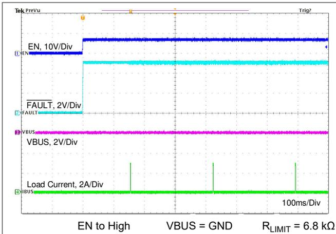
**Figure 11-26. Enable Into Short With External FET**
