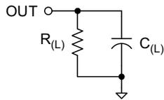
**Figure 9-1. V<sub>CONN</sub> Switch Rise-Fall Test Load Figure**
