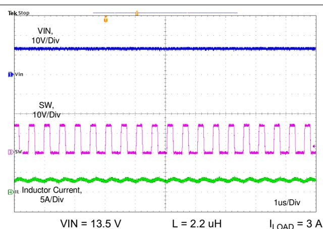
**Figure 10-9. Switching Frequency When  $R_T = 8.87\text{ k}\Omega$**
