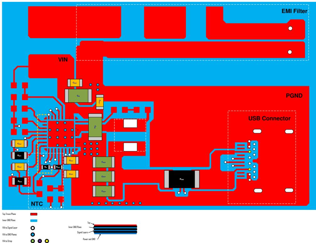
**Figure 10-31. NTC Placement Example**
