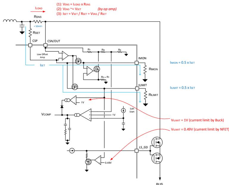
**Figure 10-15. Current Limit and Cable Compensation Circuit**
