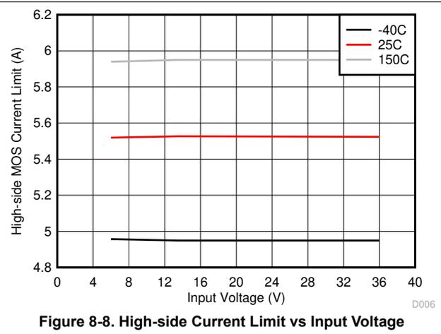
**Figure 8-8. High-side Current Limit vs Input Voltage**
