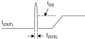
**Figure 9-3. Short-Circuit Parameters**
