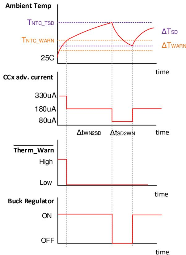
**Figure 10-29. TPS25831-Q1 Behavior When Trigger NTC Threshold**
