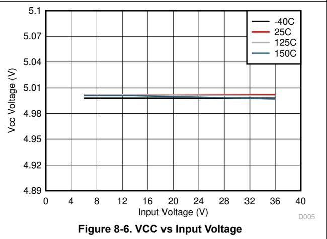
Figure 8-6. VCC vs Input Voltage
