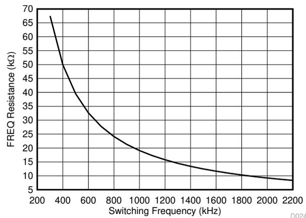
Figure 10-6. RT Set Resistor vs Switching Frequency
