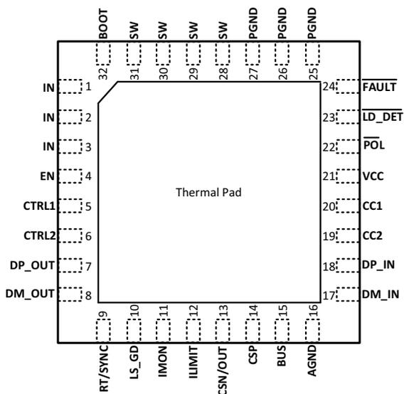
**Figure 7-3. TPS25830QCWRHBRQ1 Package 32-Pin (VQFN) Top View (2)**
