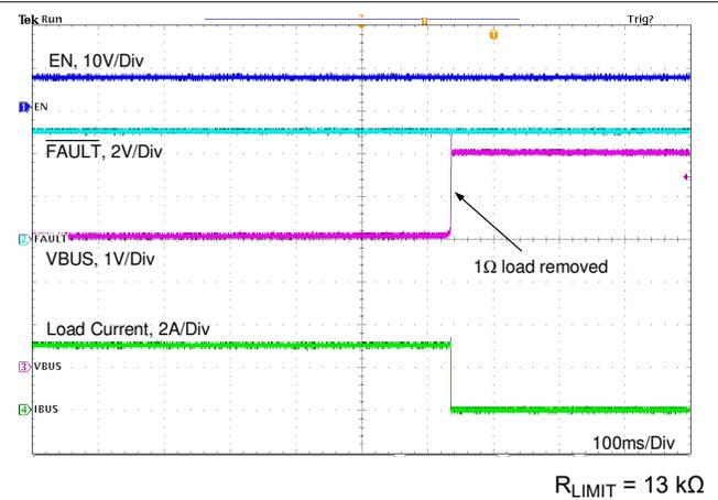
**Figure 11-25. 1-Ω Load Recovery Without External FET**
