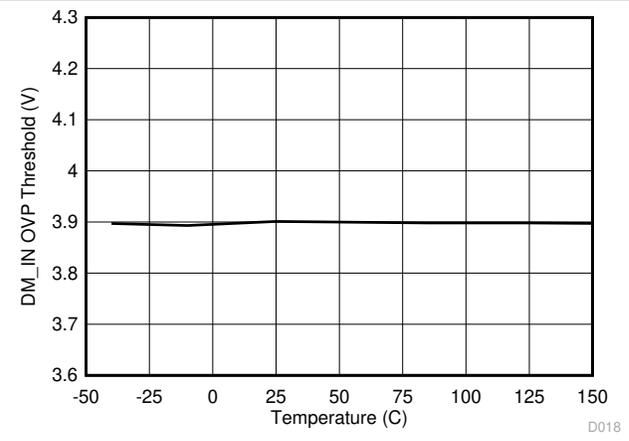
**Figure 8-22. DM\_IN Overvoltage Protection Threshold vs Junction Temperature**
