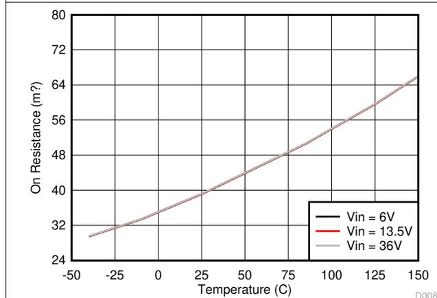
**Figure 8-9. High-side MOSFET on Resistance vs Junction Temperature**
