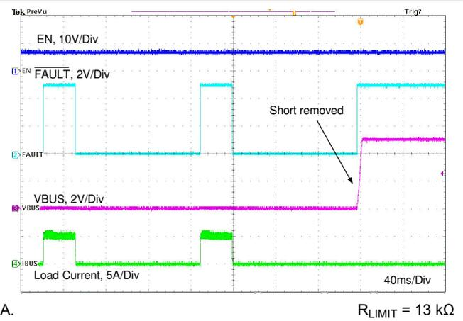
**Figure 11-23. Short Circuit Recovery Without External FET**
