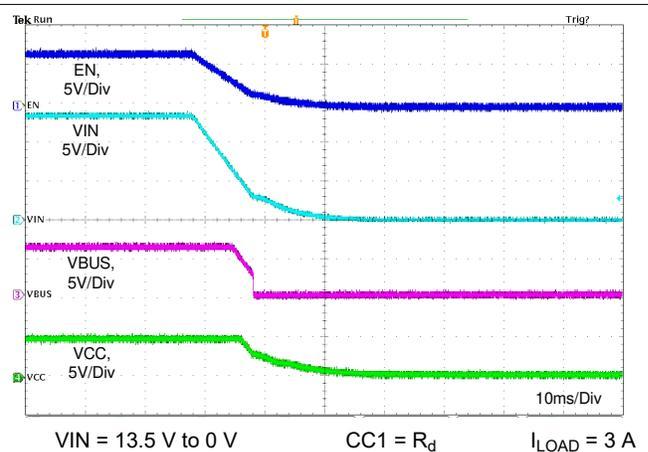
$VIN = 13.5\text{ V to }0\text{ V}$        $CC1 = R_d$        $I_{LOAD} = 3\text{ A}$
