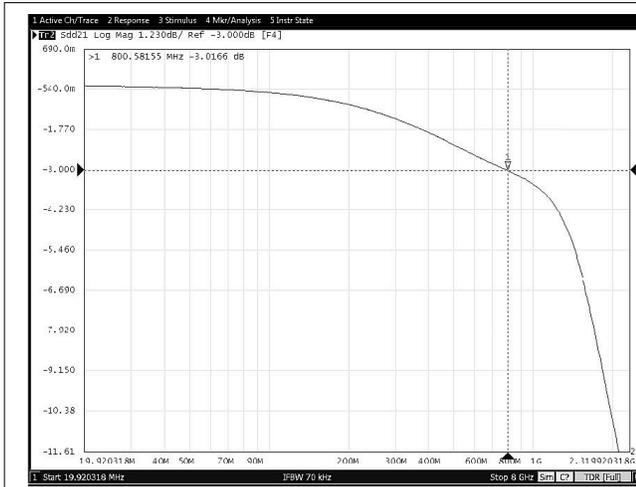
**Figure 8-31. Data Transmission Characteristics vs Frequency (TPS25830-Q1)**
