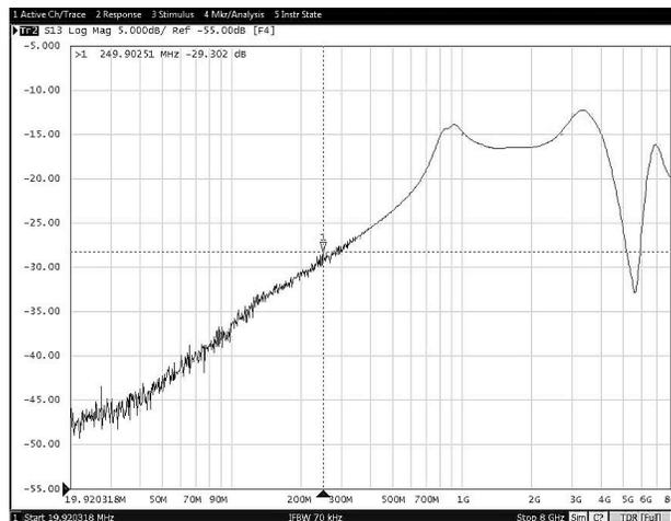
**Figure 8-33. On-State Cross-Channel Isolation vs Frequency (TPS25830-Q1)**
