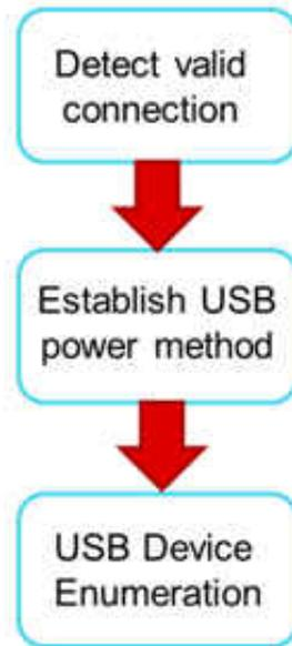
**Figure 10-24. Flow of DFP to UFP Configuration**
