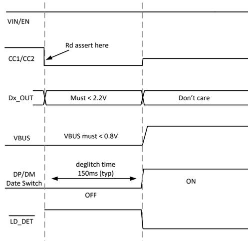
Figure 10-5. TPS25830-Q1 Pin Voltage Requirement During Rd Assert
