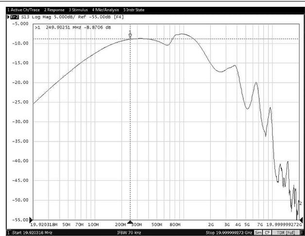
**Figure 8-32. Off-State Data-Switch Isolation vs Frequency (TPS25830-Q1)**
