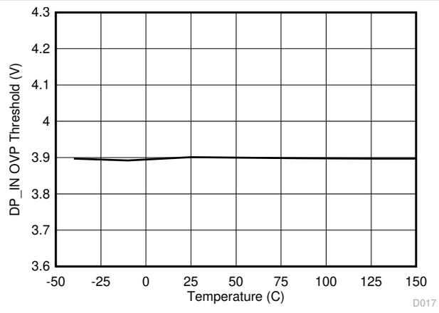
**Figure 8-21. DP\_IN Overvoltage Protection Threshold vs Junction Temperature**
