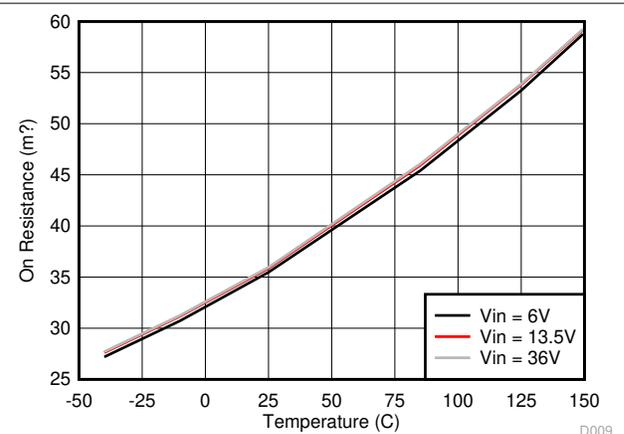
**Figure 8-10. Low-side MOSFET on Resistance vs Junction Temperature**
