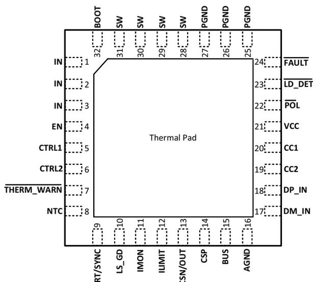
**Figure 7-4. TPS25831QCWRHBRQ1 Package 32-Pin (VQFN) Top View (2)**
