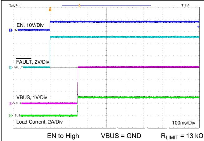
**Figure 11-24. Enable into 1-Ω Load Without External FET**
