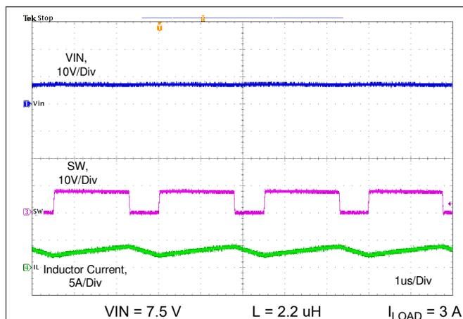
**Figure 10-8. Switching Frequency When  $R_T = 8.87\text{ k}\Omega$**
