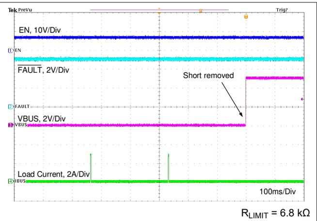
**Figure 11-27. Short Circuit Recovery With External FET**
