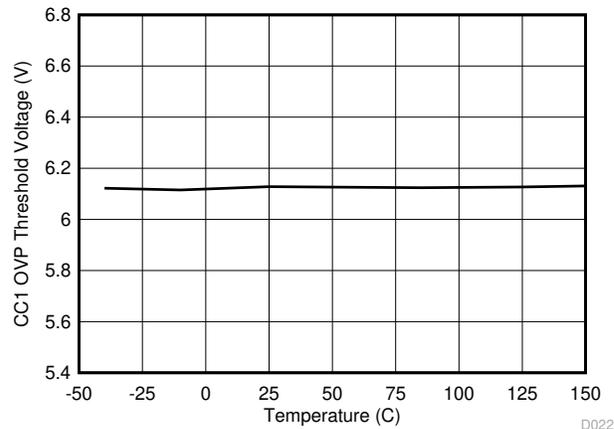
**Figure 8-26. CC1 Overvoltage Protection Threshold vs Junction Temperature**
