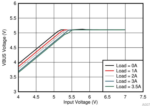
**Figure 11-12. Dropout Characteristic**
