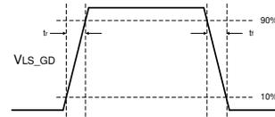
**Figure 9-4. NFET Gate Drive Rise and Fall Time**
