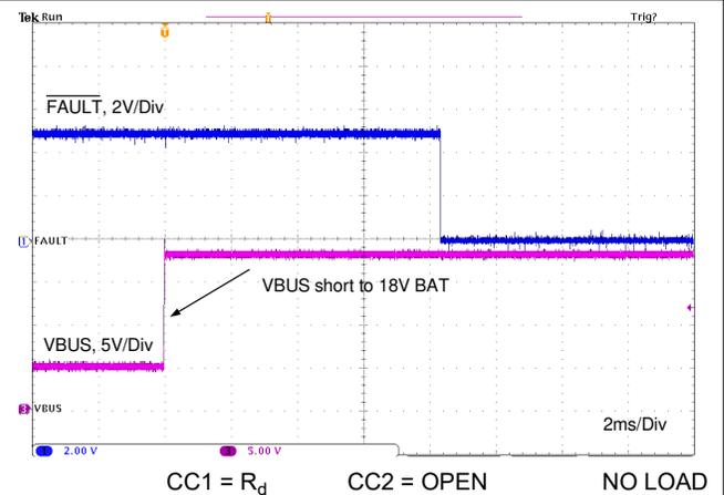
**Figure 11-31. VBUS Short to BAT With External FET**
