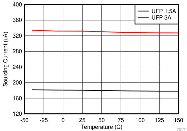
**Figure 8-25. CC Sourcing Current vs Junction Temperature**
