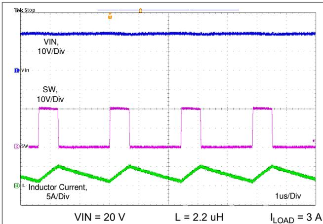
**Figure 10-10. Switching Frequency When  $R_T = 8.87 \text{ k}\Omega$**
