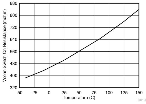
**Figure 8-23.  $V_{CONN}$  Current Limiting Switch On Resistance vs Junction Temperature**
