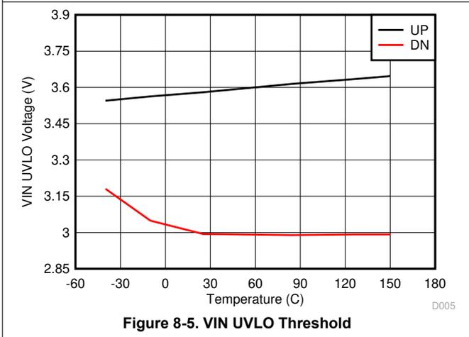
Figure 8-5. VIN UVLO Threshold
