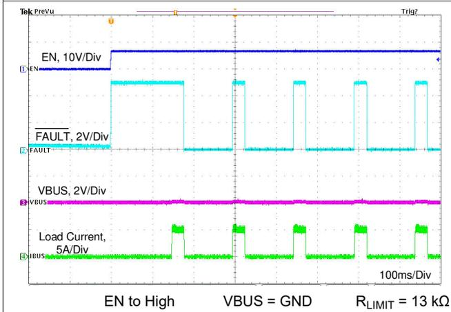
**Figure 11-22. Enable into Short Without External FET**
