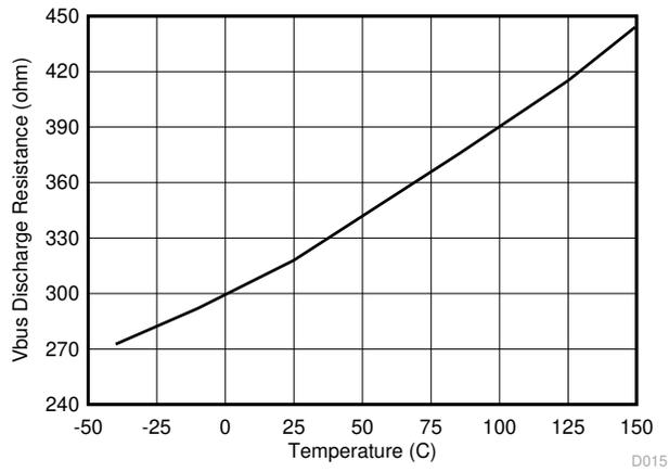
**Figure 8-19.  $V_{BUS}$  Discharge Resistance vs Junction Temperature**
