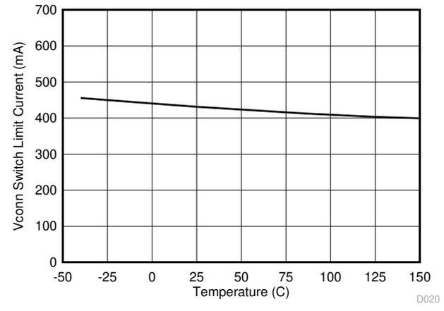
**Figure 8-24.  $V_{CONN}$  Switch Current Limit vs Junction Temperature**
