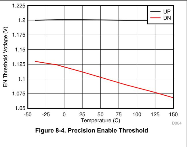
Figure 8-4. Precision Enable Threshold
