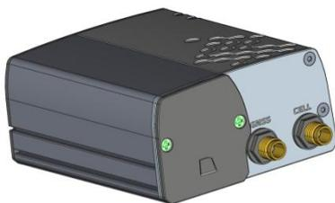
Undo the two countersunk M2 Phillips Head screws and set them aside
