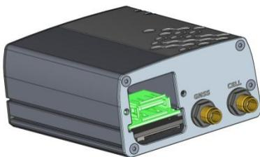
Gently push the IoT card into the slot. There should be almost no force required at this point.
