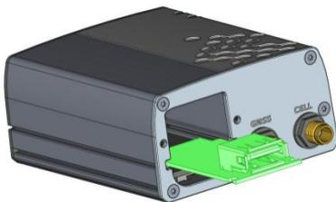
Carefully line up the IoT card with the slots in the aluminium extrusion.
