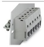
Panel feed-through terminal block, Connection method: Screw connection, Cable lug connection, Load current: 232 A, Cross section:  $35 \text{ mm}^2$  -  $95 \text{ mm}^2$ , AWG 4 - 2/0, Connection direction of the conductor to plug-in direction:  $0 \degree$ , Width: 25 mm, Color: gray
